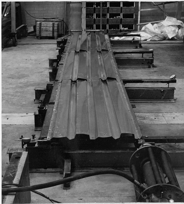
Plate (6.1) Interaction of overlapping sheets fastened in alternate troughs. The concertina action is displayed.
