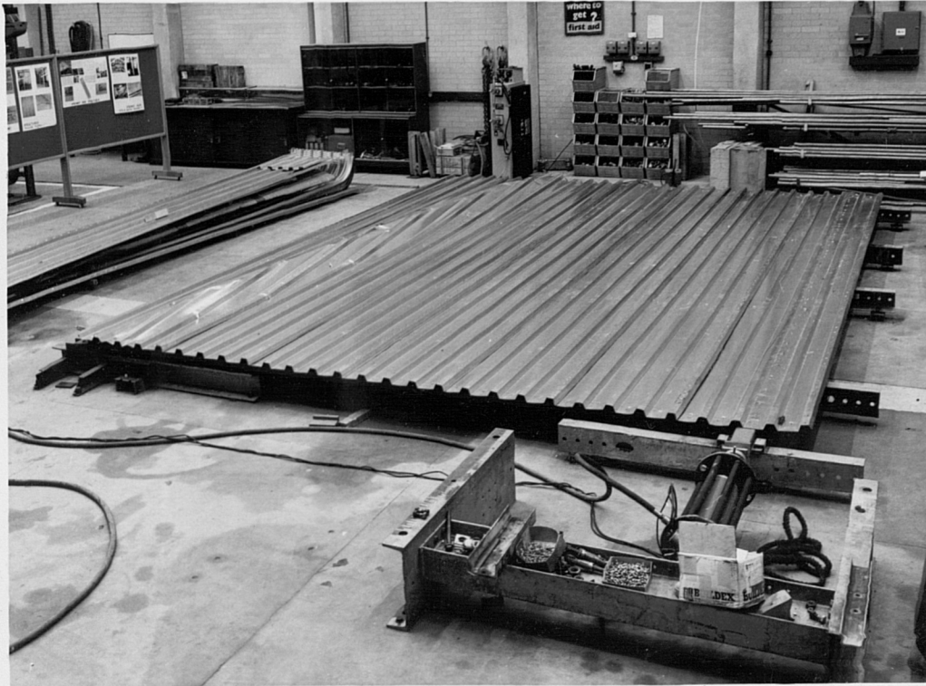
Plate (9.3) Buckling wave passes through alternate trough fastenings at two intermediate purlins
