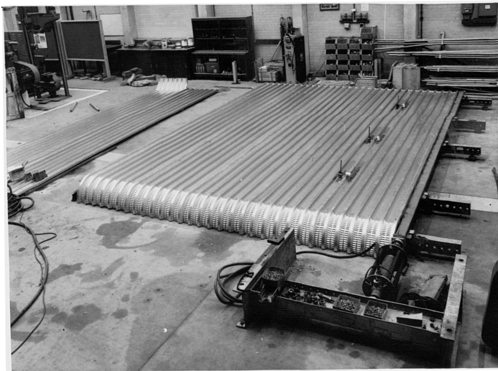
Plate (5.4) Sheeting with curved overhangs also reduce concertina action
