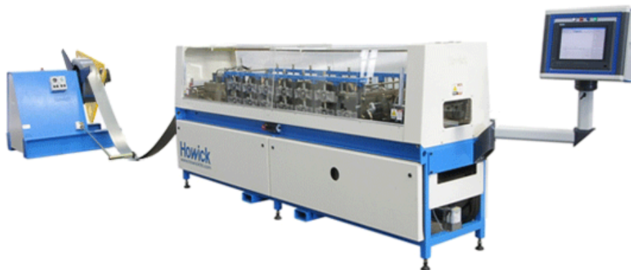
Figure 5: The Howick Framing Machine (source: Howick, 2010)
