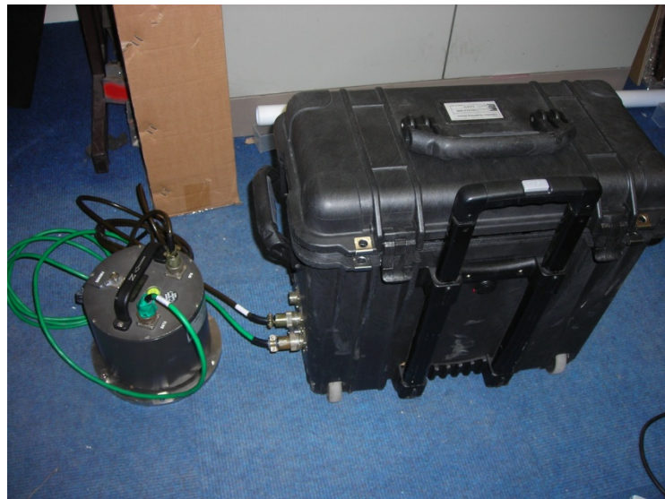
Figure 16. Guralp CMG-5TD force-feedback strong-motion accelerometer (Peris et al., 2011)
