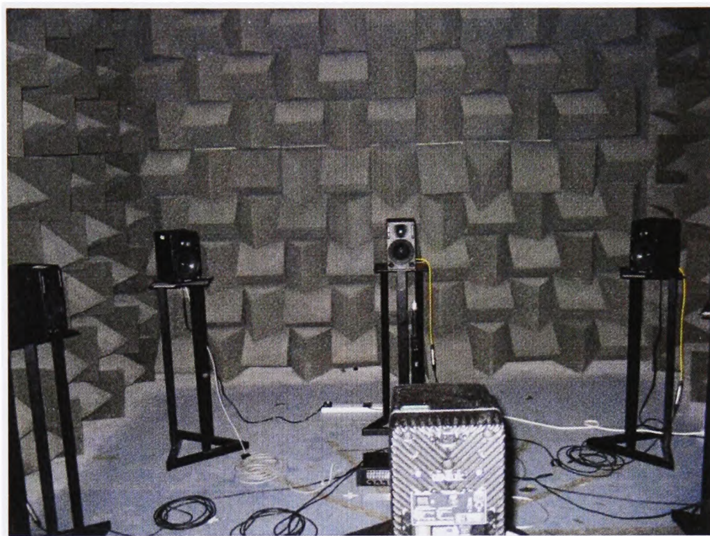
Figure 4-11 : Picture of ambisonics setup in semi-anechoic chamber
