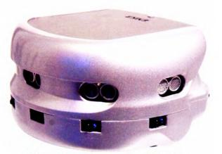
Figure 6.15: Khepera III mobile robot.
