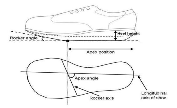
Figure 3. 1: Definition of the rocker outsole design features (rocker angles, apex position and, apex angle).
