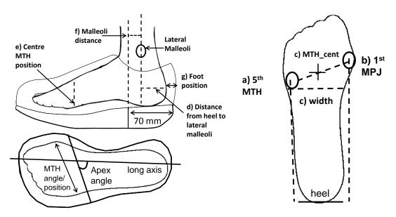
Figure 3. 5: Calculation of the foot position inside the shoe and definition of the anatomical landmarks
