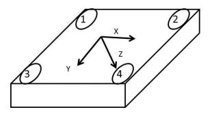
Figure 5. 7: Piezoelectric force plate schematic.
