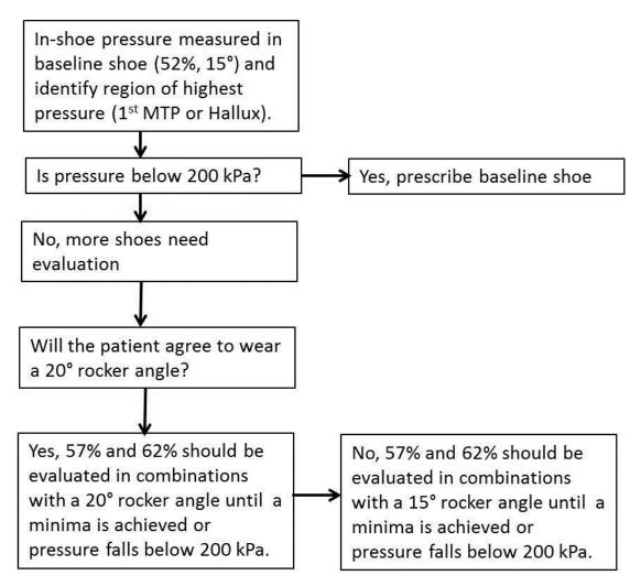
Figure 4. 21: Flow diagram of the proposed prescription method.
