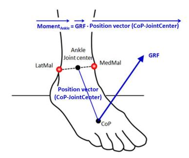
Figure 5. 10: Joint moment definition for the ankle joint.
