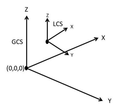
Figure 5. 5: Local coordinate system attached to a moving segment (LCS) within the global coordinate system (GCS).
