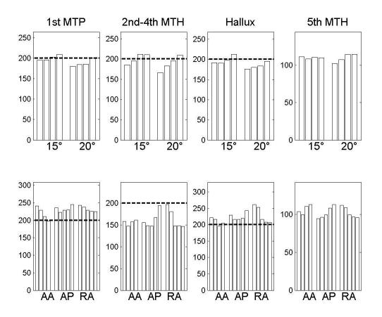
Figure 4. 20: Peak plantar pressure (kPa) for the rocker shoes from current study (top row using a 95° apex angle) in comparison to the shoes from the previous study (chapter 4) (bottom row using a 80° apex angle) for the forefoot regions (the results were recalculated using only the people with diabetes for chapter 4).
