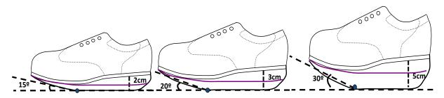
Figure 3. 20: The increase in heel height caused by increasing the rocker angle.
