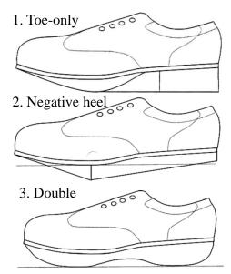
Figure 2. 3: Three different rocker sole designs, 1) toe-only, 2) negative heel and, 3) double.
