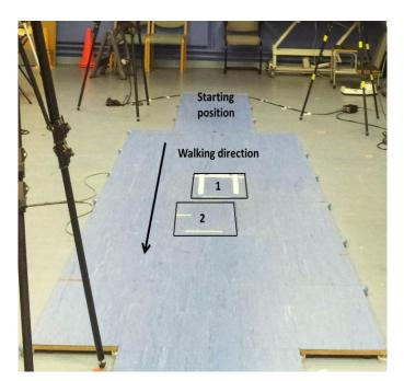
Figure 5. 6: Force plate and walkway arrangement.
