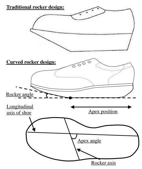
Figure 2. 4: The traditional rocker design and the curved rocker design with the three design features: 1) rocker angle, 2) apex position and 3) apex angle.
