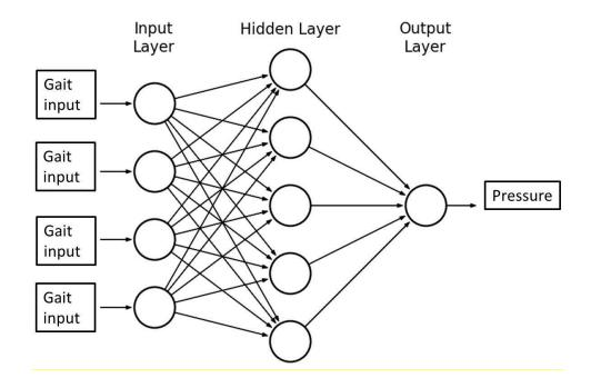
Figure 5. 11: An example of a neural network with one hidden layer (artificial neurons) Many neural networks use a number of hidden layers to increase the accuracy.
