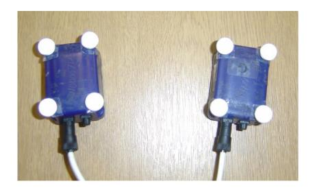
Figure 4.13: Xsens inertial sensing units with clusters of four reflective markers attached
