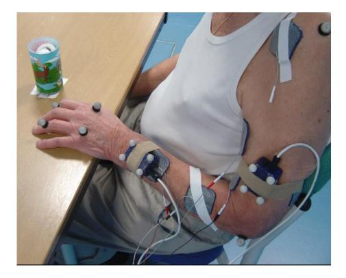
Figure 4.14: Experimental setup showing Xsens units with reflective marker clusters
