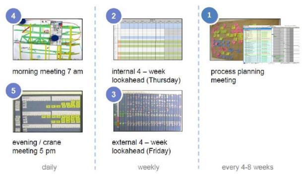
Figure 7.26: Overview of meetings as part of the LCM instantiations to power plant construction
