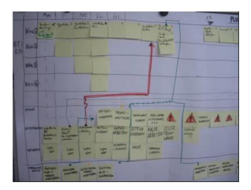
Figure 4.5: Overall Process Map (OPM): Visualising the construction process at the case study side. The interdependencies between the apartments and other areas of the building highlighted in red and green.
