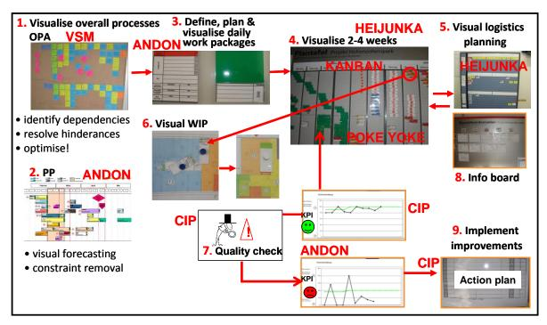
Figure 8.5: Coordinated application of visual tools from the TPS using the LCM model
