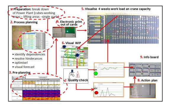
Figure 7.1: Version 3 of the LCM model - new elements highlighted in circles
