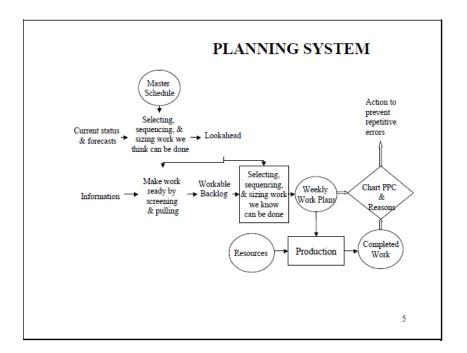
Figure 2.8 The Last Planner System with lookahead process highlighted, Ballard (2000)
