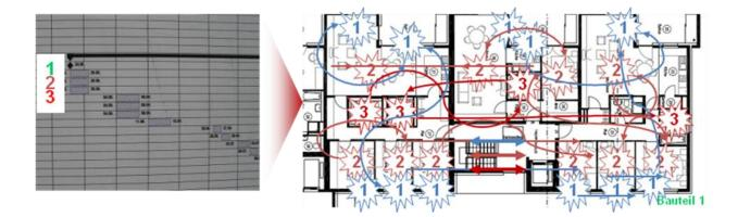
Figure 4.4: Flow of work on a daily basis (master plan left, physical work being carried out right)
