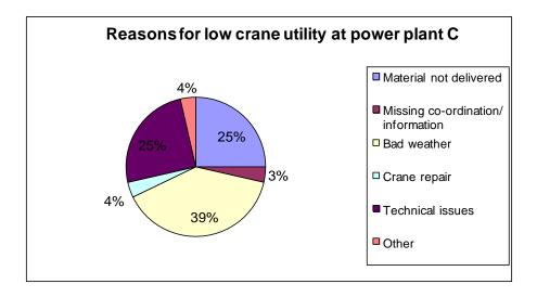
Figure E.5: Reasons for low crane utility at power plant C, Block D
