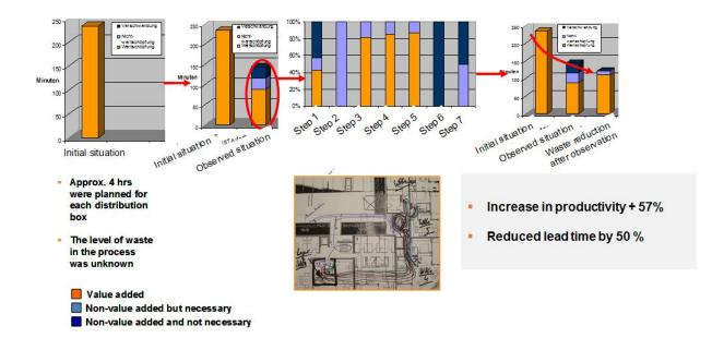
Figure C.1: Observation of the electrical assembly process
