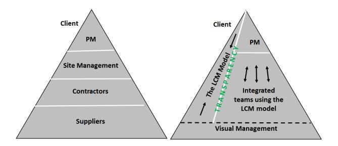
Figure 2.11: Functional orientated structure of projects (with little transparency and one-way communication, left) versus process orientated structure (using Visual Management to open up interfaces, create transparency and support two-way communication, right).
