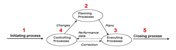
Figure 2.3: The closed loop of managerial processes in project management according to the PMBOK Guide (adapted from Koskela & Howell, 2002).
