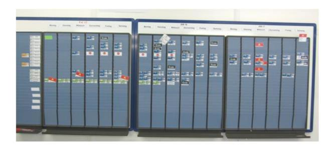
Figure 7.18: the planning board - on the x-axis the weeks and the days were shown. On the yaxis, the areas were displayed. The red problem cards can be seen in front of the work packages where they occur.
