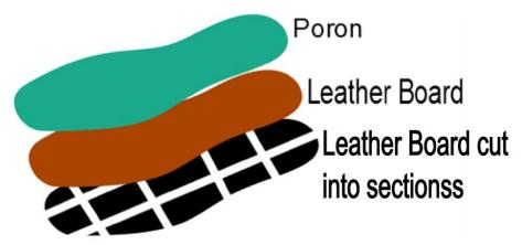
Figure 91: layers of the insoles
