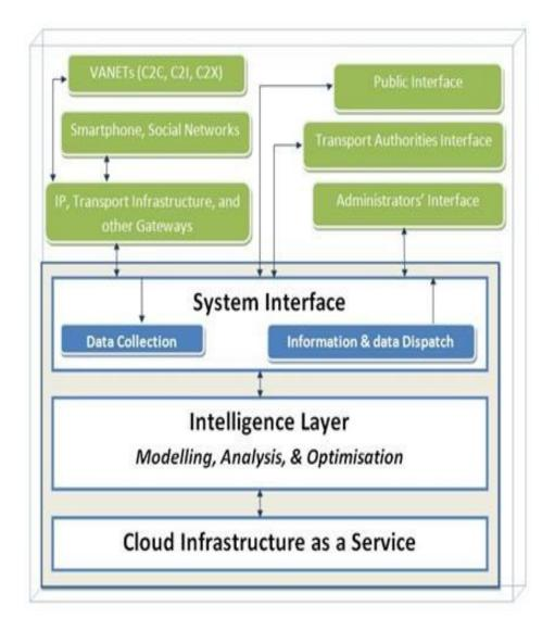
Figure 5.1 Intelligent Disaster Management System - Proposed Architecture
