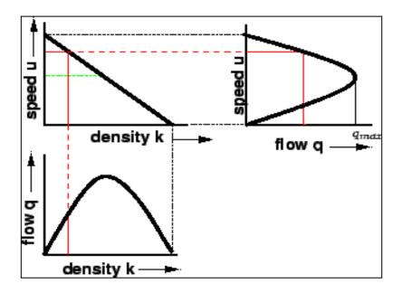
Figure 4.1 The relationships between the main basic road variables [160]
