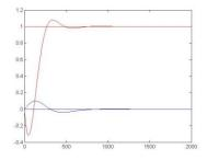
Figure 2.31: the output 1 and 2 of GA design full controller with weight factor=10
