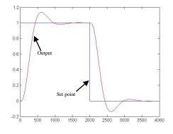
Figure 3.5: The output with Actuator 2 failure
