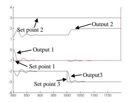
Figure 4.39: The output 1 and 3 under control for multi input multi output override control system
