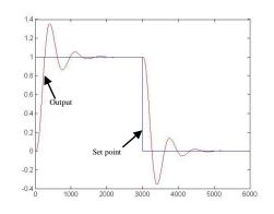
Figure 3.21: The output with Actuator 2 failure
