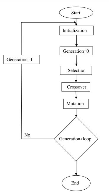
Figure 2.2: The basic cycle of genetic algorithm
