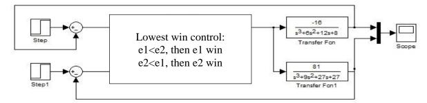
Figure 4.5: One input two output override control system with negative sign in steady-state transfer function matrix
