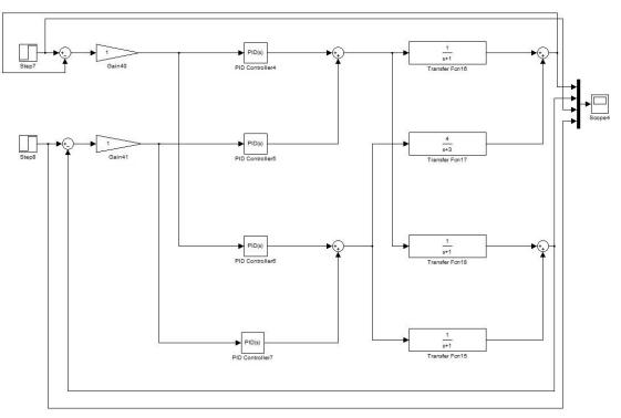
Figure 2.52: Square multivariable control system transfer function
