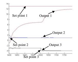
Figure 4.40: The output 2 and 3 for multi input multi output override control system
