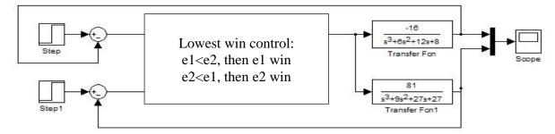
Figure 4.12: One input two output override control system
