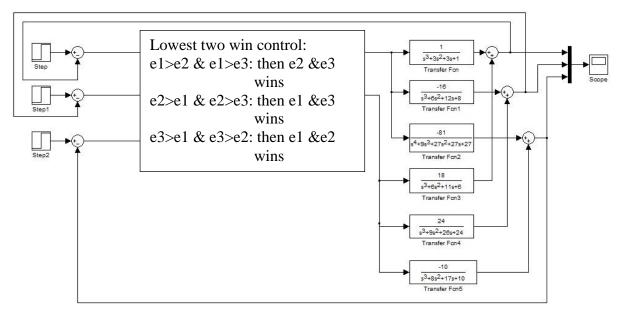
Figure 4.26: Multi input multi output override control system block diagram
