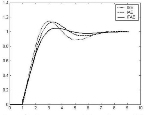
Figure 2.1: Closed loop step response resulted from applying proposed PID parameters
