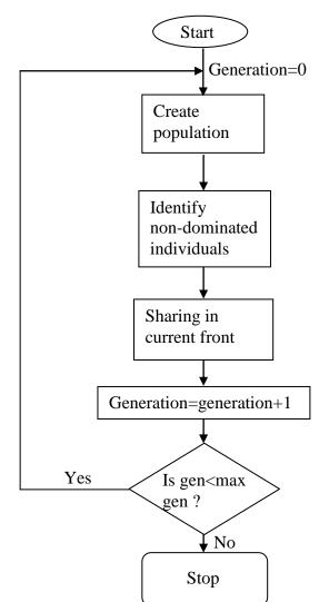
For multi-objective GA, the Pareto optimal method is used. And the chart of this method is shown below:
