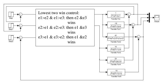
Figure 4.28: Multi input multi output override control system block diagram As figure 4.24 shows, the six transfer functions are
