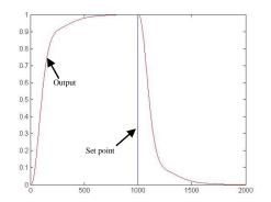
Figure 3.10: The output with Actuator 1 failure
