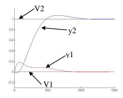
Figure 2.46: the output 1 of GA design the full controller with the set-point changing
