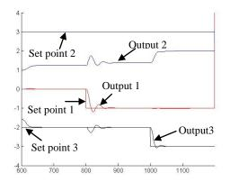
Figure 4.24: The output 1 and 3 under control for multi input multi output override control system
