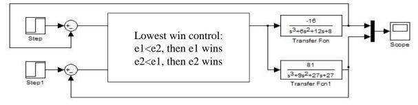
Figure 4.8: One input two output override control system As figure 4.8shows, the two transfer functions are
