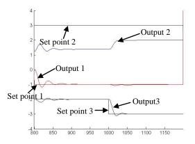
Figure 4.33: The output 1 and 3 under control for multi input multi output override control system
