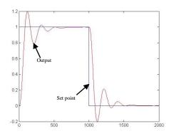
Figure 3.17: The output with Actuator 1 failure
