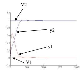
Figure 2.16: the output 2 of GA design  $k_{p1}$ ,  $k_{p2}$ ,  $k_{p3}$ ,  $k_{p4}$ ,  $k_{i1}$ ,  $k_{i2}$ ,  $k_{i3}$  and  $k_{i4}$  wi th the set-point changing and interaction
