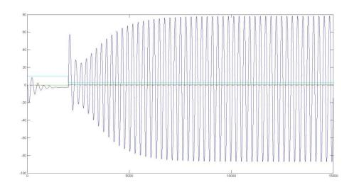
However, for another range of set points the system could start to limit cycle. For this reason it is important to know the exact range which the override system will not limit cycle.
