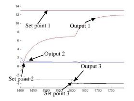
Figure 4.37: The output 2 and 3 for multi input multi output override control system
