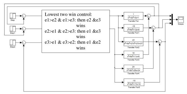
Figure 4.14: Multi input multi output override control system block diagram
