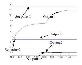
Figure 4.34: The output 2 and 3 for multi input multi output override control system
