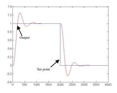
Figure 3.4: The output with Actuator 1 failure
