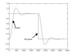
Figure 3.24: The output with Actuator 2 failure
