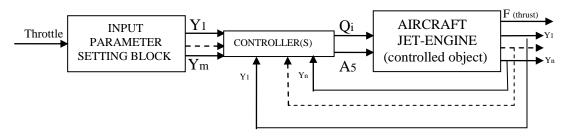
Figure 4.1: Aircraft engine's automatic control system
