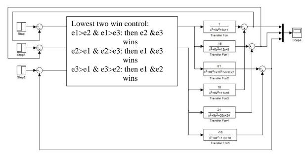
Figure 4.22: Multi input multi output override control system block diagram
