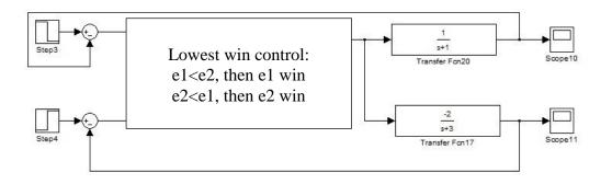
Figure 4.2: override control when loop one under control
