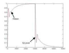
Figure 3.20: The output with Actuator 1 failure
