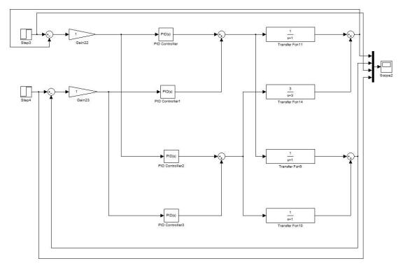
Figure 2.33: Square multivariable control system transfer function
