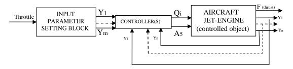
Figure 1.2: Aircraft engine's automatic control system
