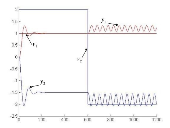
Figure 4.7: System output of the one input two output override control system with negative sign in steady-state transfer function matrix
