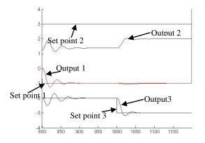
Figure 4.36: The output 1 and 3 under control for multi input multi output override control system
