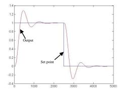
Figure 3.11: The output with Actuator 2 failure
