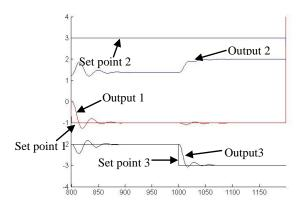
Figure 4.30: The output 1 and 3 under control for multi input multi output override control system
