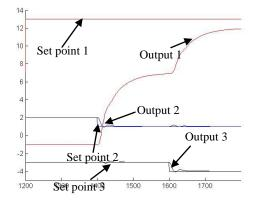
Figure 4.25: The output 2 and 3 for multi input multi output override control system
