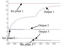
Figure 4.31: The output 2 and 3 for multi input multi output override control system
