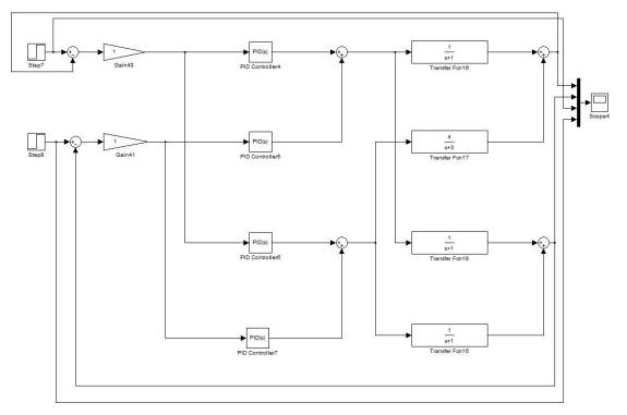
Figure 2.38: Square multivariable control system transfer function
