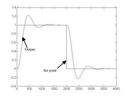
Figure 3.18 The output with Actuator 2 failure
