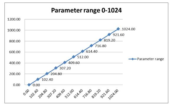
For example, in GA, each parameter could be coded by a 10 bits binary number, the parameter range is from 0 to 1024. So the decode and scale the binary number will be:
