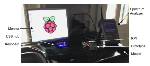
Figure 4.1 Experimental Set-up with Spectrum Analyzer (from I-r monitor, keyboard, powered USB hub, RPi, prototype, spectrum analyzer, mouse)
