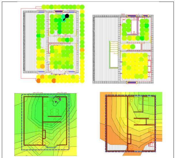
Figure 5.18 Comparison of modelled signal strength (bottom) and actual signal strength (above) at the Salford Energy House, ground floor (left) and first floor (right)
