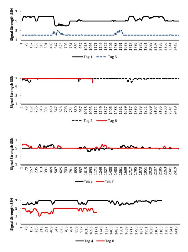
Figure 5.57 Comparison of resulting signal strengths from co-located tags
