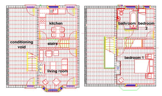
**Figure 4.3 Layout of the Salford Energy House ground floor (left) and first floor (right)** As can be seen from the floorplans in Figure 4.3 the house is of a traditional twoup two-down design. There is an additional full-height and 1/3-width house built adjacent to the property (the conditioning void) to correspond to the energy house being an end terraced dwelling.
