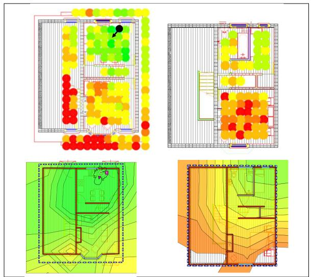
Figure 5.4 Comparison of the spectrum analyzer results (top) and Ekahau modelling of the Energy House, ground floor (left) and first floor (right)
