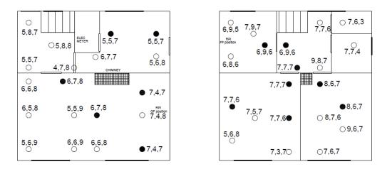
Figure 5.62 The triple point signal strength combinations
