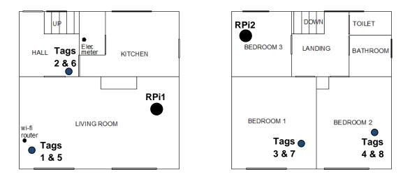
Figure 5.33. The RPi and tag locations during the Environmental Effects Test 2
