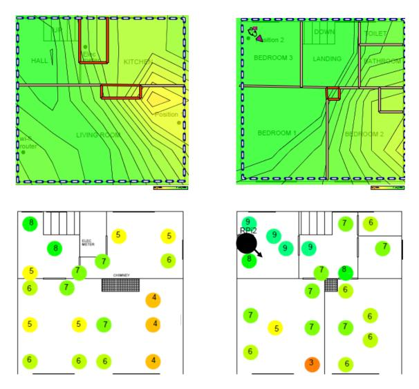
Figure 6.2 The simulated signal contour map (above) and actual signal strength results (bottom) from triple point position 2 at Home1, ground floor (left) first floor (right)
