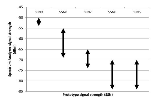
Figure 5.19. Comparison of spectrum analyzer and prototype signal strength
