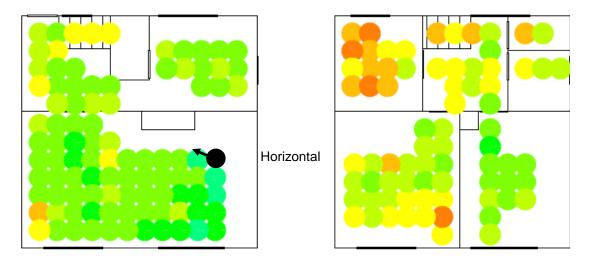
Figure 5.20 Home1 Test 4 with the RPi placed in the living room, horizontal and directed towards the front door. Ground floor (left) and first floor (right)
