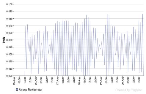
Figure 3.1 Hourly Energy Consumption pattern over several days for a refrigerator
