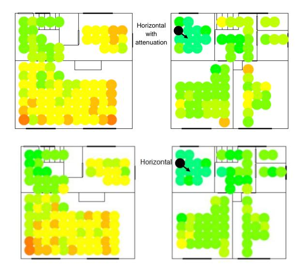
Figure 5.27. Resulting heatmaps from Test 11 with attenuation (top) and Test 6 without attenuation (bottom)
