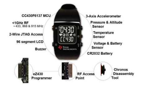
Figure 3.2 The Texas Instruments eZ430-Chronos Development Tool (image from Texas Instruments)
