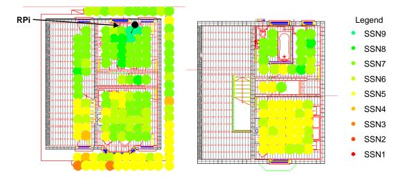
Figure 4.16. Example of a heatmap from a test at the Salford Energy House (ground floor (left) and first floor (right)). The RPi position and reader direction indicated as in the kitchen and towards the opposite corner of the house.
