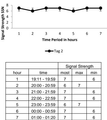
Figure 5.36. Resulting signal strength of Tag 2 during Environmental Effects Test 2
