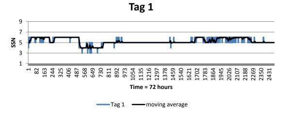
Figure 5.48 Tag 1 signal strength over 72 hours in the Environmental Effects Test 3
