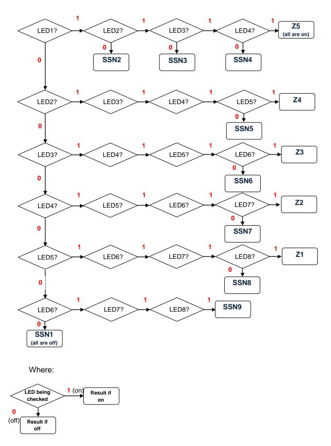
The decision flowchart of the Python programme designed to carry out the least number of checks of the LEDs in order to correctly determine the Signal Strength Number (SSN)
