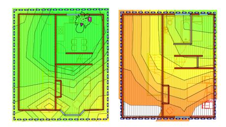
Figure 4.17. Heatmap of the Salford Energy House ground floor (left) and first floor (right) using Ekahau ESS Pro 7.6.4 software.
