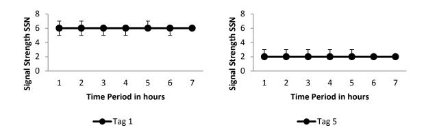
Figure 5.43. Tag 1 and Tag 5 signal strength behaviour at the same location during Environmental Effects Test 2
