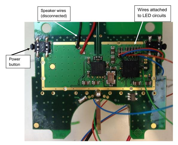
Photograph of the reverse of the Loc8tor handheld unit showing the wires connected to LED circuits on the Loc8tor handheld unit.
