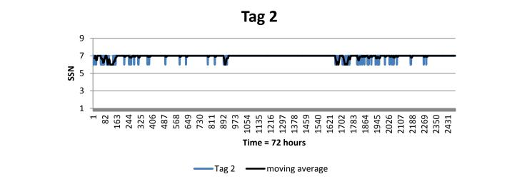
Figure 5.49 Tag 2 signal strength over 72 hours in the Environmental Effects Test 3 Figure 5.49 presents the resulting signal strength from Tag 2.The signal from Tag 2 was less disrupted than Tag 1 and tends to remain at SSN7 throughout the three days of the test.
