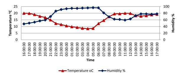
Figure 5.29 The humidity and temperature observations during the period of Environmental Effects Test 1
