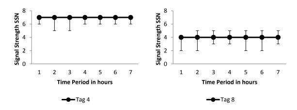
Figure 5.46. Tag4 and Tag8 signal strength behaviour at the same location during Environmental Effects Test 2
