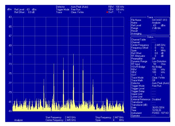
Figure 4.15 Output from the spectrum analyzer showing a peak tag signal at -71dBm during tests at the Salford Energy House
