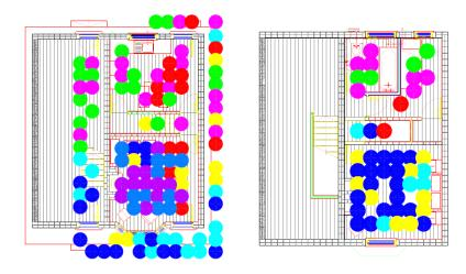
Figure 5.10 all the locations of the most commonly occurring signal strength combinations from the Energy House tests 2 and 3.
