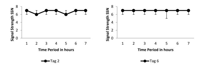
Figure 5.44. Tag 2 and Tag 6 signal strength behaviour at the same location during Environmental Effects Test 2
