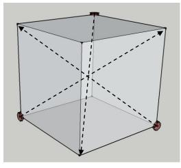
Figure 4.9 The ideal locations for readers when using triple points to locate tags within the cube.
