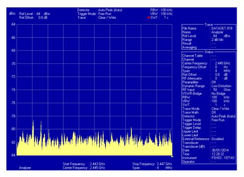
Figure 5.6 Example of Spectrum Analyzer with no distinguishable signal strength visible above the background
