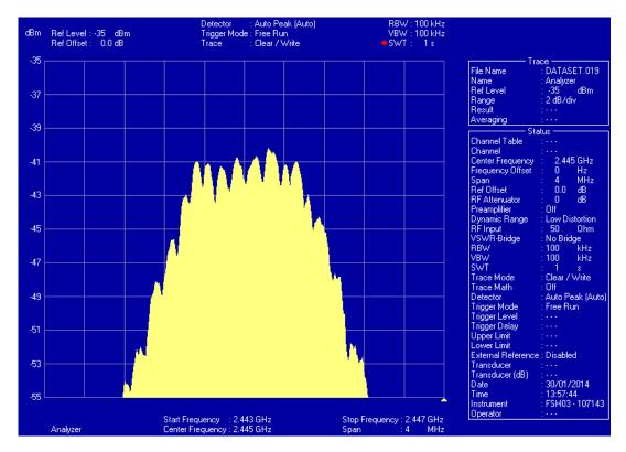
Figure 5.5 Example of the broad spectrum signal from the Loc8tor handheld unit to activate a tag
