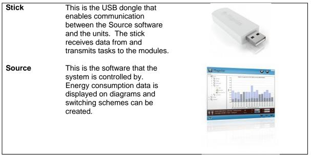
The Elements that make up the Plugwise Energy Management and Control System. (images from www.plugwise.com)
