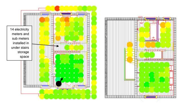
Figure 5.8. RPi results from Test 2 at the Salford Energy House, ground floor (left) and first floor (right)
