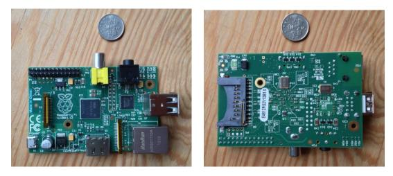
Figure 3.7 Top (left) and underside (right) of the Raspberry Pi (RPi) computer, with a UK 5 pence coin for scale
