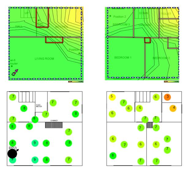
Figure 6.3 The simulated signal contour map (above) and actual signal strength results (bottom) from triple point position 3 at Home1, ground floor (left) first floor (right)
