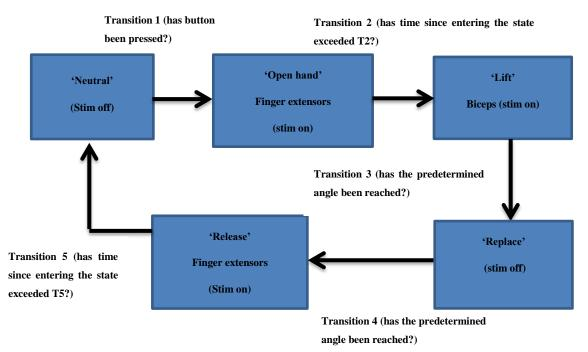
Figure 3.3: Example FSM for drinking from a glass. Boxes represent the states and T1-T5 the transitions between states.
