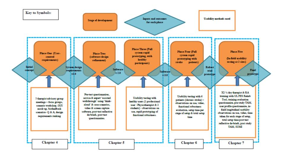
Figure 8.1: UL FES Rehab Tool development lifecycle, inputs and outputs and the associated usability evaluation methods for phases 1-5, based on Money et al, (2011).
