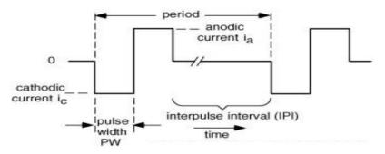
Figure 2.7: Typical waveform for FES (Merrill et al., 2005). The narrow pulse width is indicated PW. The interpulse interval (IPI) is the time between pulses.
