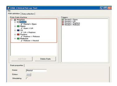
Figure 3.2: The CST software interface. The upper section of the screen highlighted in red, displays a tree-view structure and finite state machine example for the drinking from a glass task. The labels attached to the arrows (x,y,t -state transitions)) indicate the inputs that were necessary to detect a 'trigger'. X and Y signify angle triggers, T = a timed trigger'. State machines are explained further in chapter 3.
