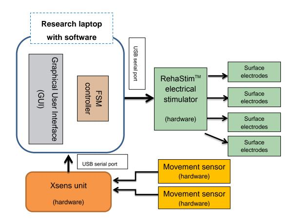
Figure 3.4: Graphical representation of the laptop with GUI, RehaStim<sup>™</sup> (FES unit) and surface electrodes, the inertial sensor system (Xsens) with 2 inertial measurement units (each comprising a 3 axis accelerometer, 3 axis gyroscope and 3 axis magnetometer).
