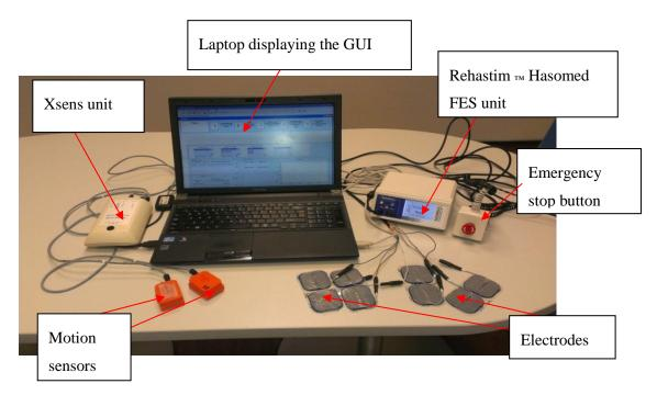
Figure 7.1: The final prototype UL FES Rehab Tool – software and hardware components
