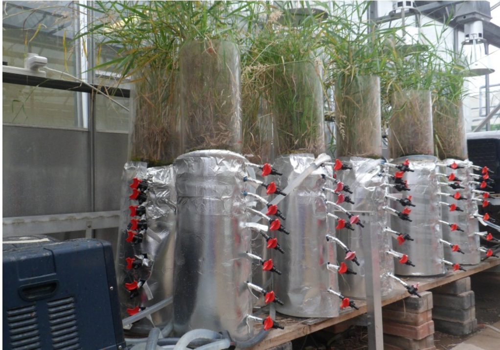
Figure 3.1 Laboratory set-up of the vertical-flow constructed wetlands
