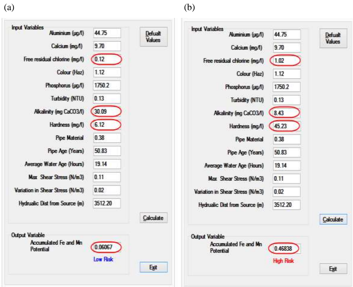
Figure 5.17 Screen shots of the developed software to show the effect of chemical oxidation on Fe and Mn accumulation potential in WSZ5
