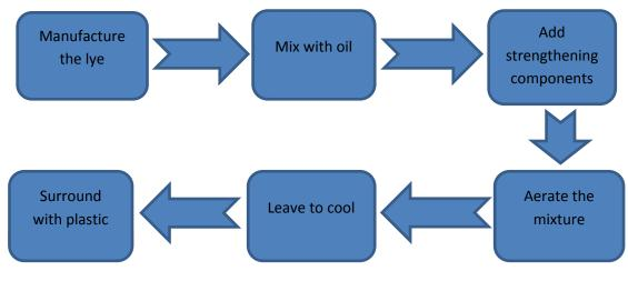
Figure 3.15: Process Diagram Showing Steps of Soap Material Development
