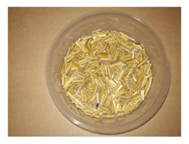
Figure 3.26: Straw Cut to 10mm – 15mm
