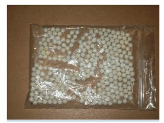
Figure 3.29: 10mm PEHD Hollow Spheres
