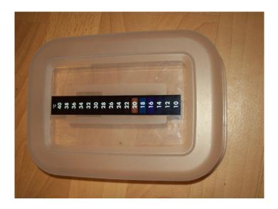
Figure 4.9: Flexible Adhesive Strip Thermometer with Plastic Case
