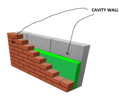
Figure 7.2: Cavity Wall Construction
