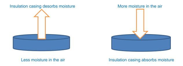
Figure 7.3: Insulation Casing before Reaching a State of Moisture Equilibration
