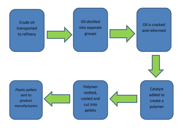
Figure 2.1: Flow Diagram Showing the Oil Refining Process
