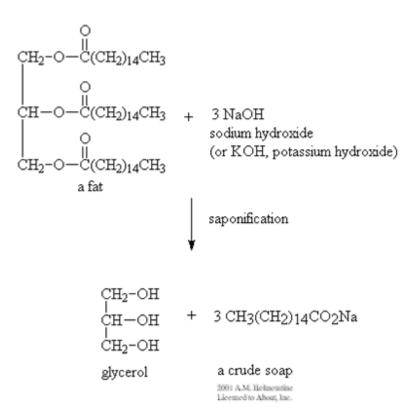
Figure 3.20: Saponification Chemical Reaction
