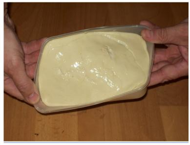
Figure 3.22: Waste Engine Oil Set to a "Blancmange" State
