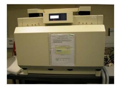
The Thermal Measurement Laboratory is a UKAS accredited laboratory. We are not UKAS accredited for the measurements detailed in this report. However, the FOX 603 apparatus was calibrated against manufacturers Certified Reference Material and against in-house UKAS accredited EN 12667 guarded hot plate apparatus with calibration traceable to National Standards.
