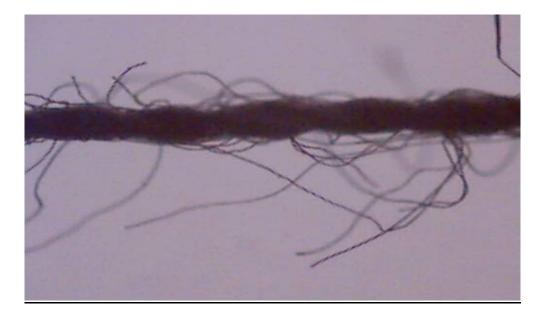
Figure 4.5: Structure of Cotton Thread (Anon.)
