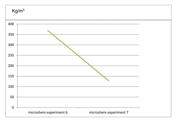
Figure 5.4: Graph Showing how Increasing Void Size Decreases Density
