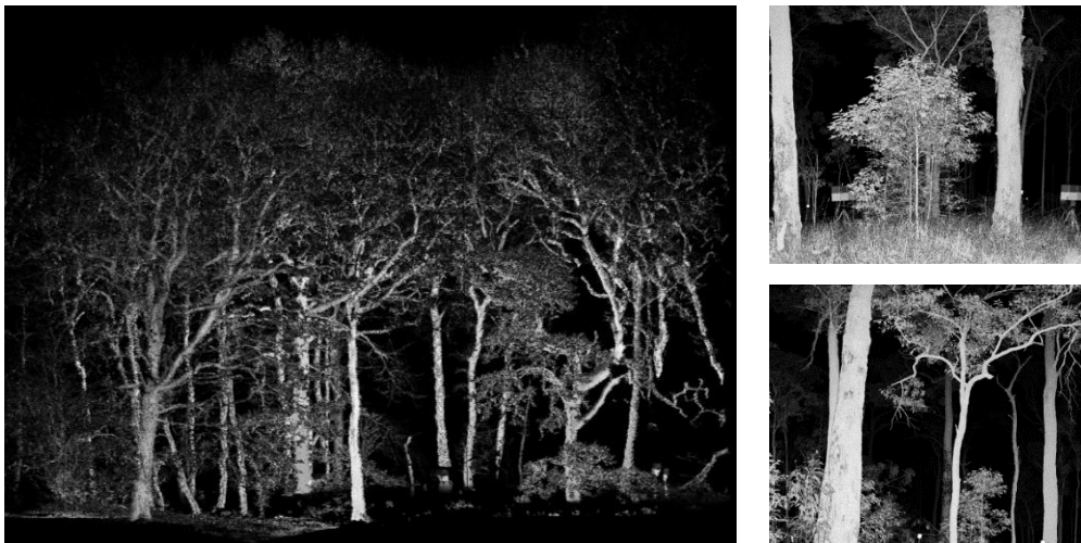
Figure 4.1. Examples of a 3D point cloud from SALCA at high resolution (0.06° in azimuth and 0.06° in zenith), plotted in 3D (left image) and 2D (right images). Datasets are from the \lambda 1545nm laser and are coloured by raw intensity (white is high intensity, dark grey is low intensity, black is no returns).
