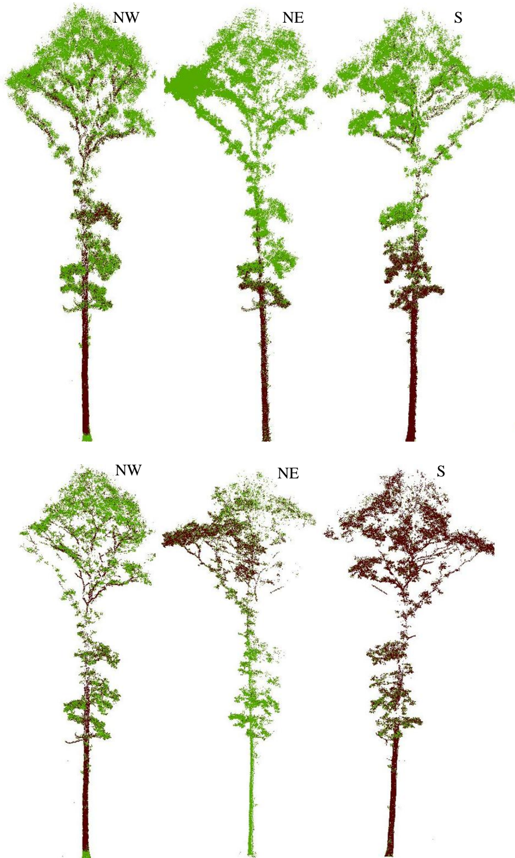
Figure 5.24. Point clouds for Tree 03 classified into 'leaf' or 'wood' using a 1545nm threshold of 0.29 (top) NDI threshold of 0.1 (bottom), for all three scanning positions. Images show leaf-on where green points have been allocated to 'leaf' category and brown points allocated to 'wood'.
