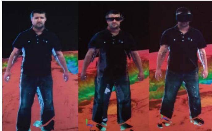
Fig. 11. This figure demonstrates the problem of occlusion (for the viewer) when using various display devices. Left: no stereo (full facial expressions); centre: stereo glasses (eye gaze and some facial features obscured) and right: HMD (most of the face obscured, identification of facial expressions not possible).(Fairchild et al., 2015)
