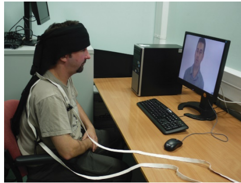
Fig. 24. Participant environment. The participant is sat facing a desktop machine that is running the sender movies in E Prime. The participant is wearing an fNIRS sensor with a scarf wrapped around it to ensure light did not affect the data captured.
