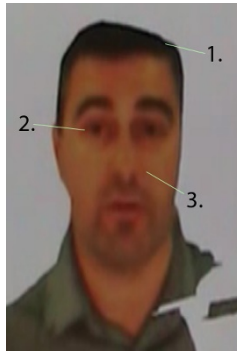
Fig. 26. Screen shot of virtuality avatar illustrating: 1. Slicing. 2. Lack of Concavities. 3. The droop effect.
