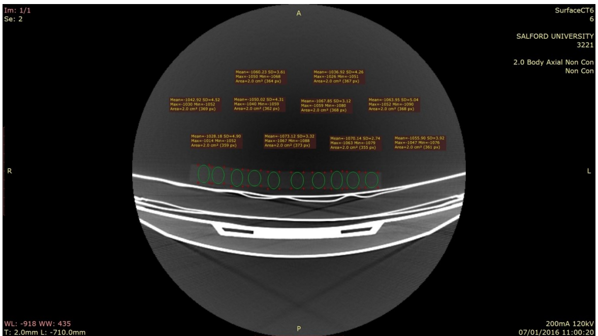
Figure 6:3: A CT image showing how the mean Hounsfield unit (HU) for the foam was calculated
