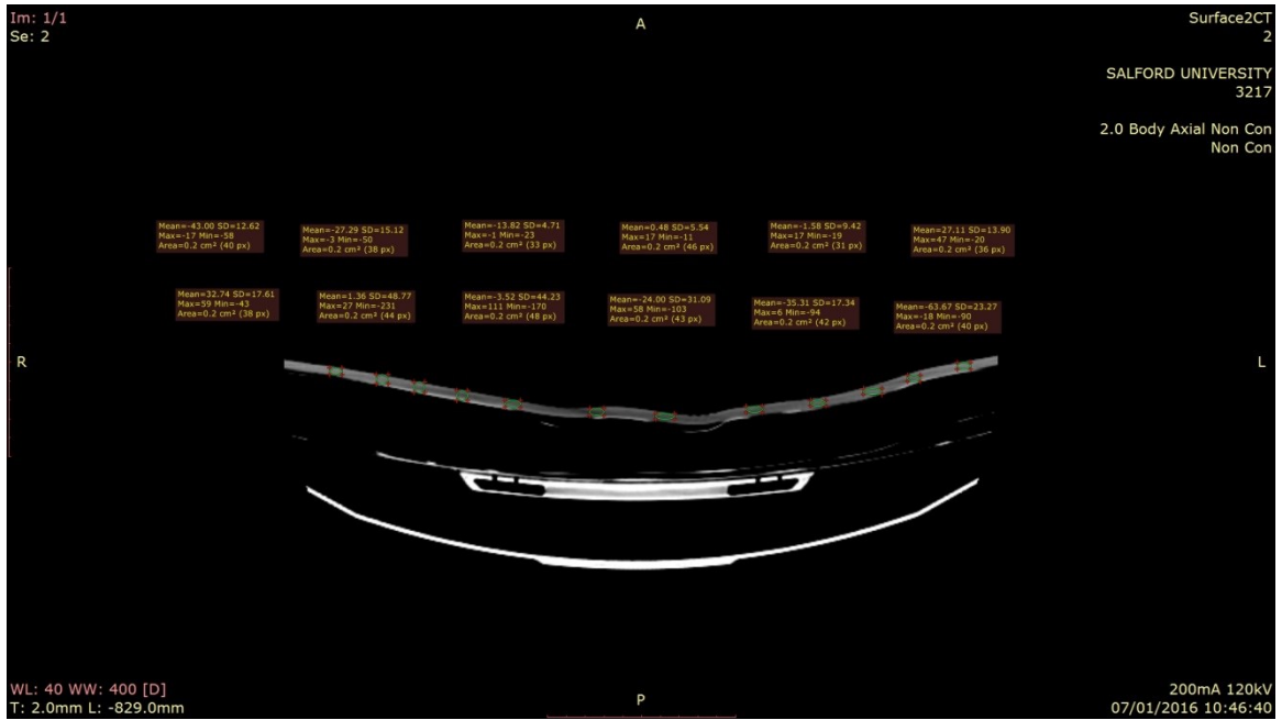
Figure 6:2: A CT image showing how the mean Hounsfield unit (HU) for the silicone gel overlay was calculated
