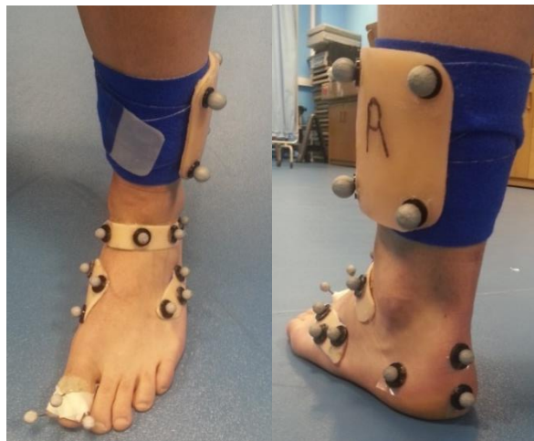
Figure 8.4: Location of the different reflective markers used to define and track foot and ankle movement
