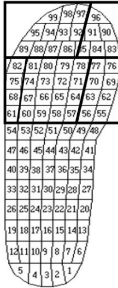
Figure 7.2: Different areas defined on the Pedar mask used in the study
