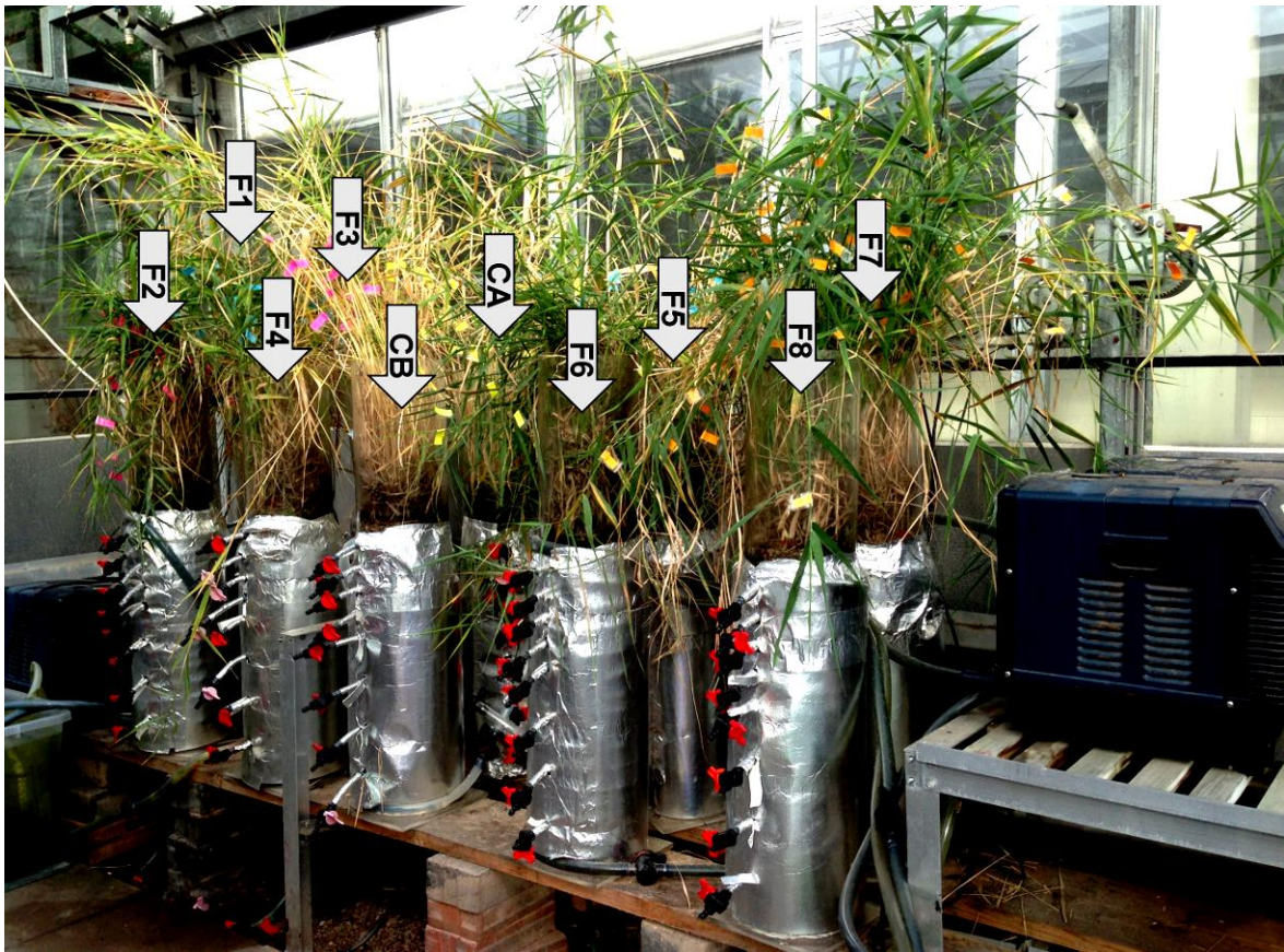
Figure 3.1: Laboratory set-up of the vertical-flow constructed wetlands in the greenhouse.
