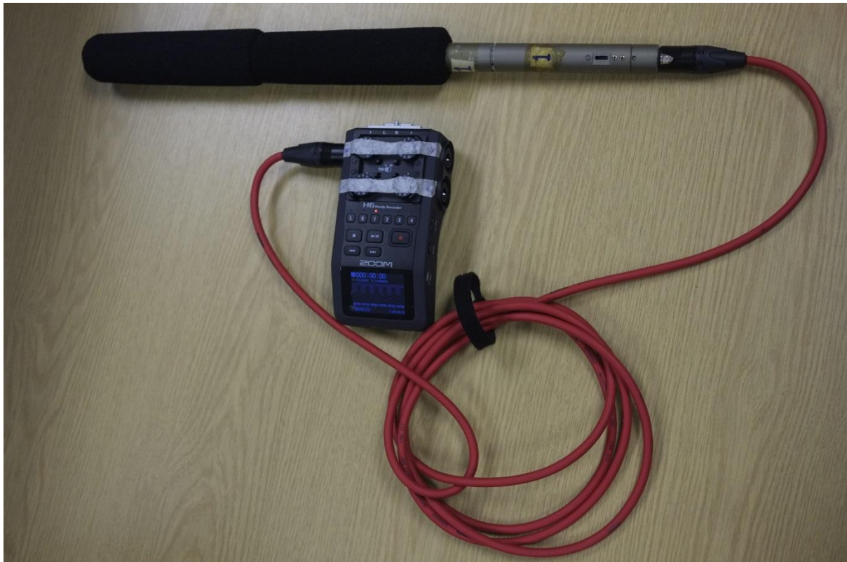
Figure 6-14 Audio-Technica AT-815A and Zoom H6 Used in Sound Object Recording
