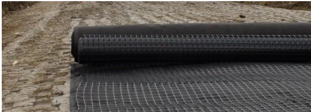
Figure 12.6: An example of Geogrid material
