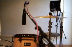
Figure 48: Overheads - Coles ribbon microphones positioned behind the player
