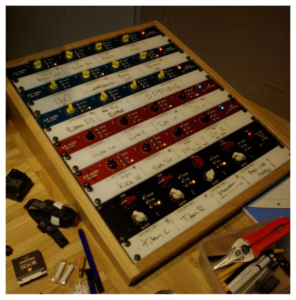
Figure 68: Microphone preamplifiers - marked each mic / D.I
