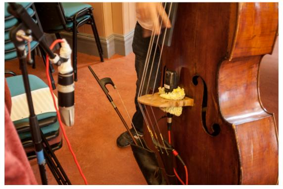
Figure 17: Bass microphone placement
