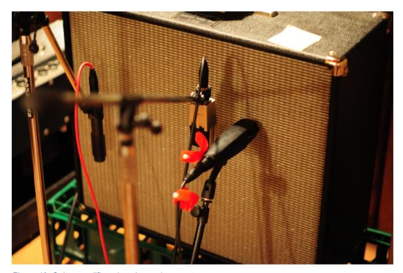
Figure 40: Guitar amplifier microphone placement
