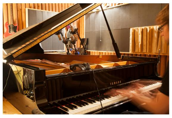
Figure 76: Final piano microphone configuration - ORTF 414s and NOS Peluso C12s
