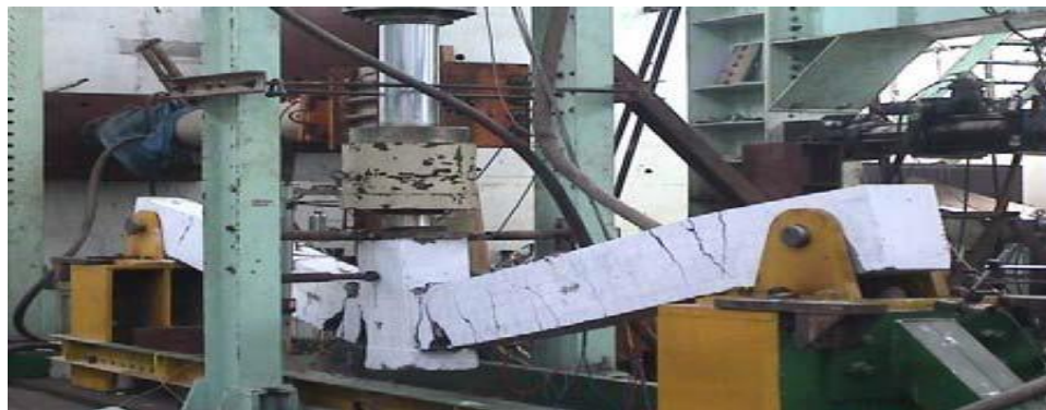
Figure 2-10 Photograph of test setup (Wei-jian and Qing-feng 2008)
