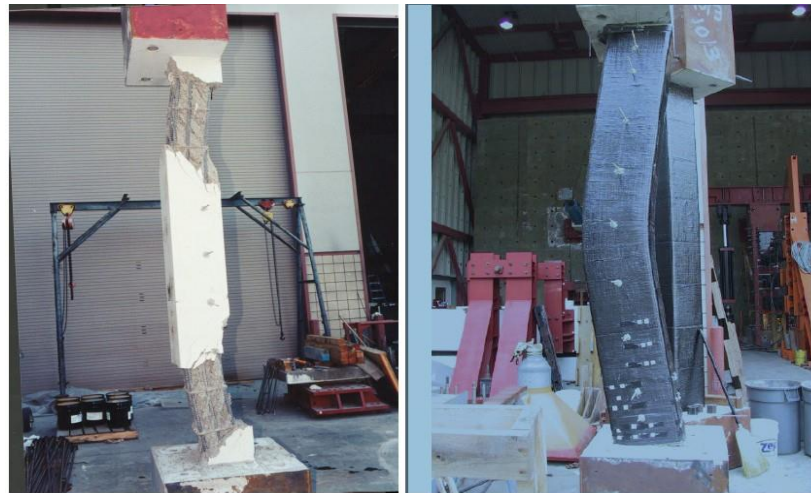
Figure 2-41 Composite wrap for reinforced concrete column (Crawford, 2002)
