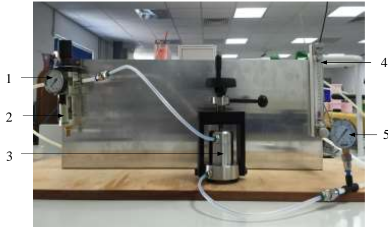
1- Upstream pressure (P2), 2- In-line-Air regulator, 3- Fancher core/sample holder, 4- Air flow meter, 5- Downstream pressure (P1)
