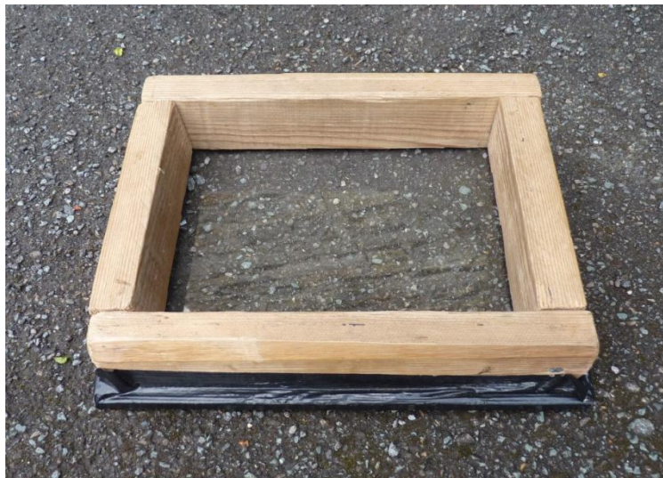
Figure 8: Glass fitted to a frame on which newts were placed before photographing them from below.
