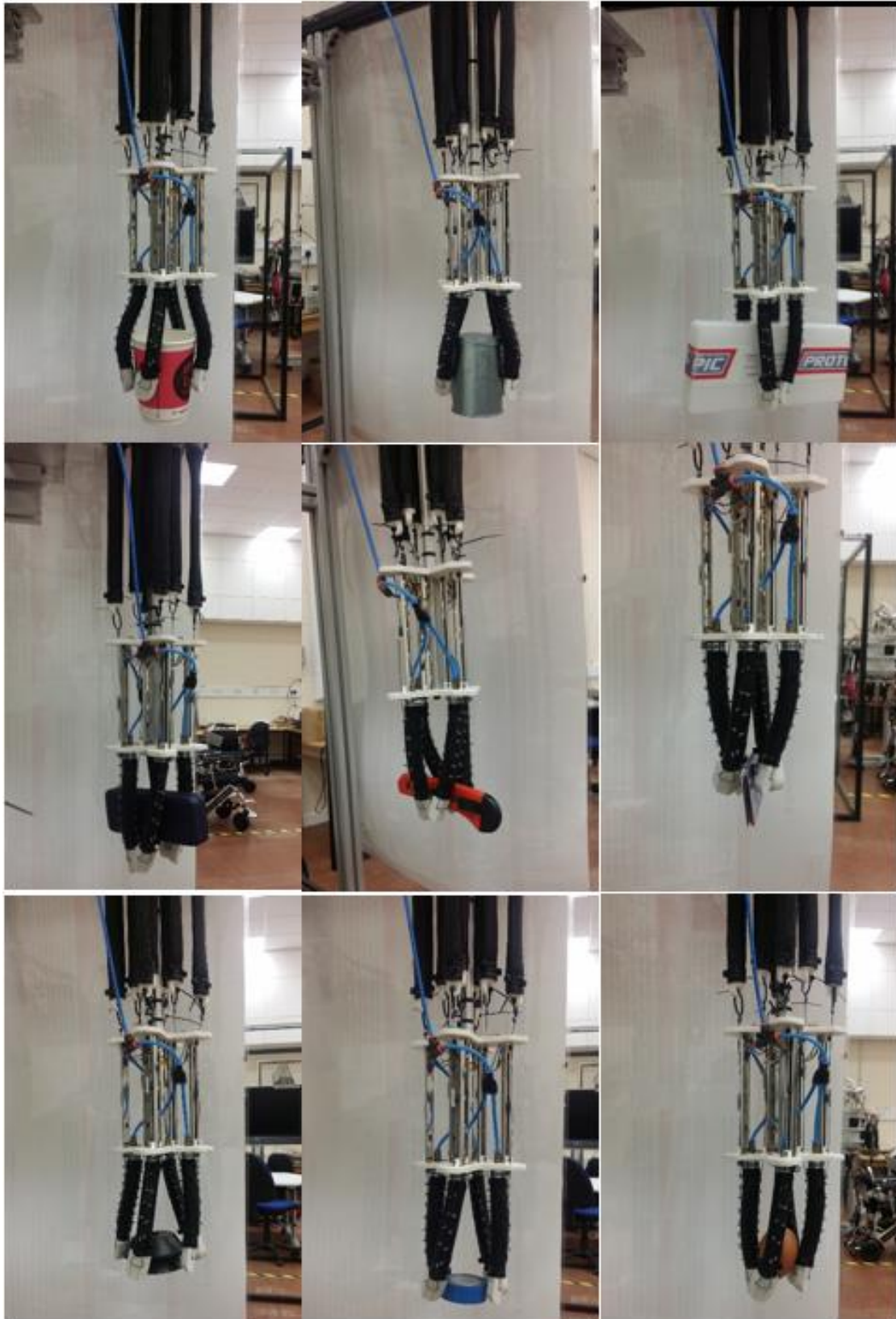
Figure 5-5: Four-fingered soft robot end effector grasping sample products.
