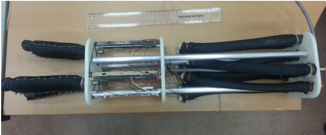
Figure 4-13: The overall actual construction of the three-fingered soft robot end effector.
