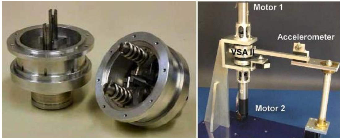
Figure 2-8: Improved VSA prototype and an experimental setup of the improved VSA in one-link robot arm (Schiavi, R., et al., 2008).
