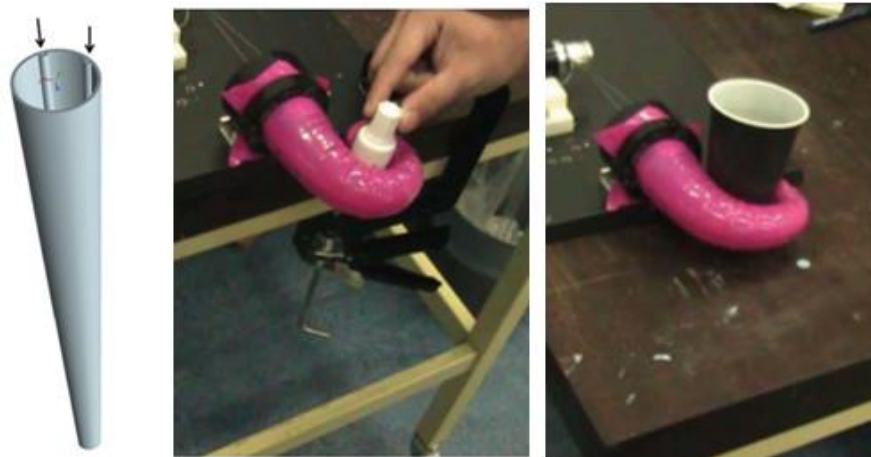
Figure 2-27: Variable compliance soft arm grasping capabilities (Giannaccini, M., et al., 2013).
