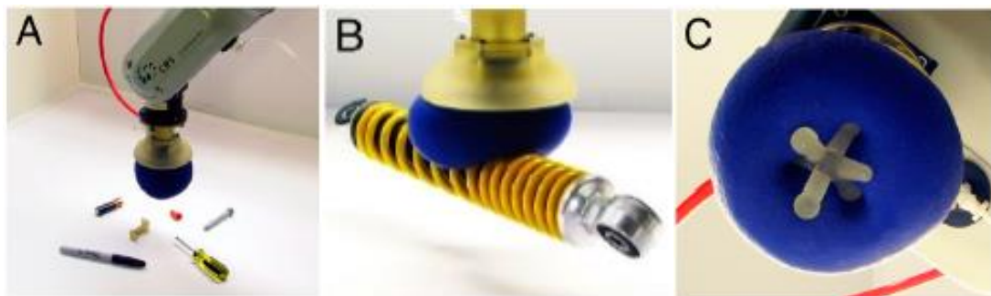
Figure 2-43: Universal unlimited DOF gripper. (A) Jamming-based universal gripper attached to a fixed-base robot arm. (B) Picking up a shock absorber coil. (C) View from the underside (Brown, E., et al., 2010).
