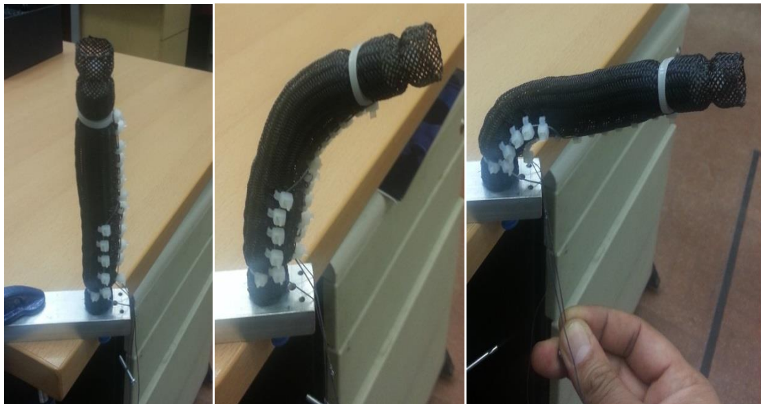
Figure 4-3: Continuum finger using pneumatic muscle actuator and tendon cables.
