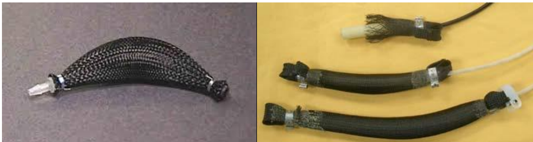
Figure 2-14: Left extensor and right contractors pneumatic muscle actuators.
