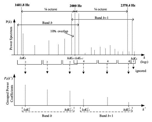
Figure 9: Grouping of power coefficients within 2 bands around 2kHz.
