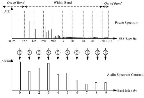
Figure 8: ASE extraction from power spectrum.
