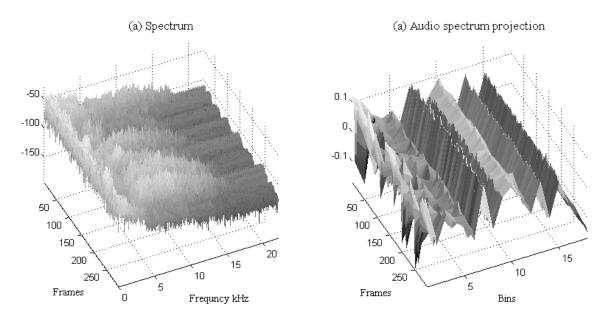
Figure 15: ASP of a speech signal (a) Signal spectrum (b) ASP feature of size 18.
