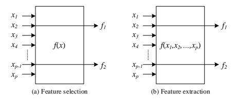
Figure 25: Dimensionality reduction using (a) feature selection, (b) feature extraction.
