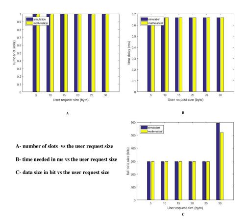
Figure B-5 Comparison Between The Mathematical Results and Simulation Result for Downlink with SF=4
