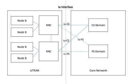
Figure 3-17 Iu Interface Between the Core Network and UTRAN
