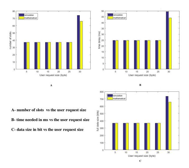
Figure B-4 Comparison Between The Mathematical Results and Simulation Result for Uplink with SF= 256
