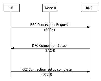
Figure 3-16 RRC Connection Establishment
