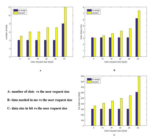
Figure C-1 Comparison Between Simulation Results of The Standard and The New Design for Uplink SF= 32
