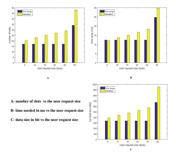
Figure 7-10 Comparison Between the Results of The 3GPP and The New Design for the Uplink SF= 128
