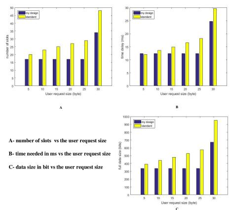
Figure C-3 Comparison Between Results of The Standard and The New Design for Uplink SF= 128
