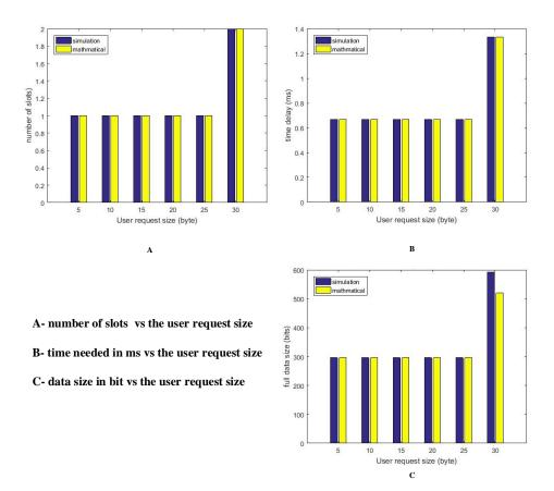
Figure B-7 Comparison Between The Mathematical Results and Simulation Result for Downlink with SF=16
