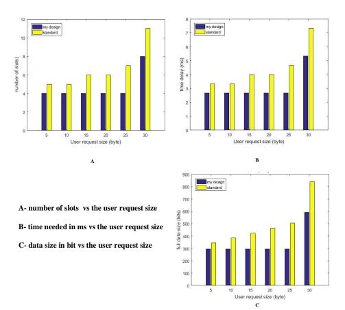
Figure C-9 Comparison Between Results of The Standard and The New Design for Downlink SF= 64
