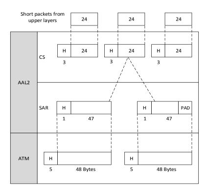
Figure 3-21 AAL2 and ATM Layers Structure
