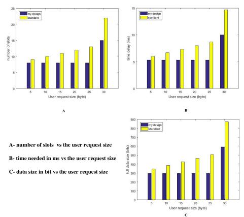
Figure C-10 Comparison Between Results of The Standard and The New Design for Downlink SF= 128
