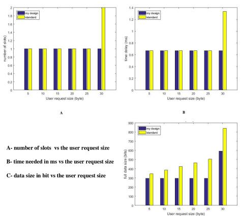
Figure C-6 Comparison Between Results of The Standard and The New Design for Downlink SF= 8
