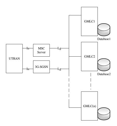
Figure 5-9 Core Network with Multiple GMLCs
