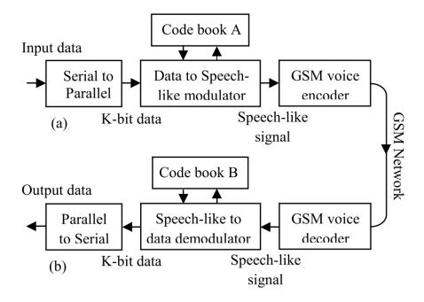
Figure 4-3 Overall Modem Structure (a) Transmitter (b) Receiver [95]
