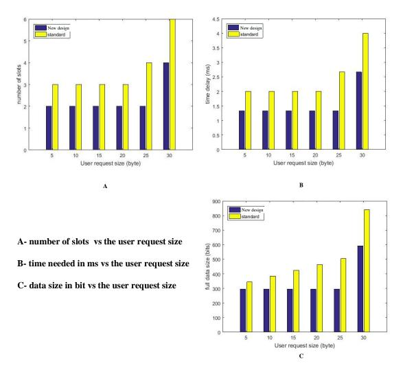
Figure 7-11 Comparison Between The Results of The 3GPP and The New Design for The Downlink SF= 32
