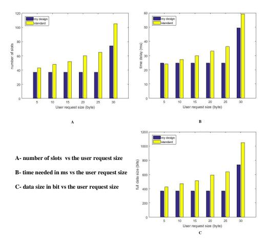
Figure C-4 Comparison Between Results of The Standard and The New Design for Uplink SF= 256
