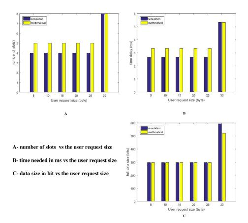
Figure B-9 Comparison Between The Mathematical Results and Simulation Result for Downlink with SF=64
