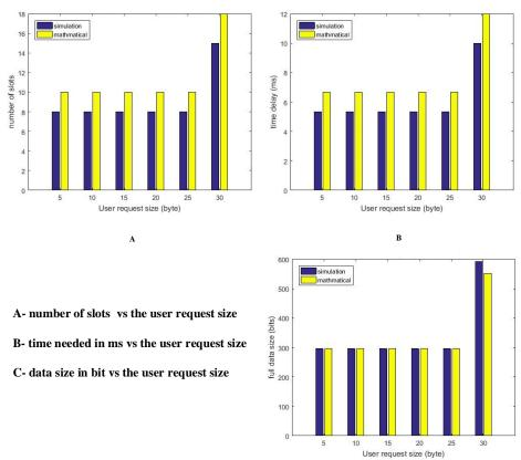
Figure B-10 Comparison Between The Mathematical Results and Simulation Result for Downlink with SF=128
