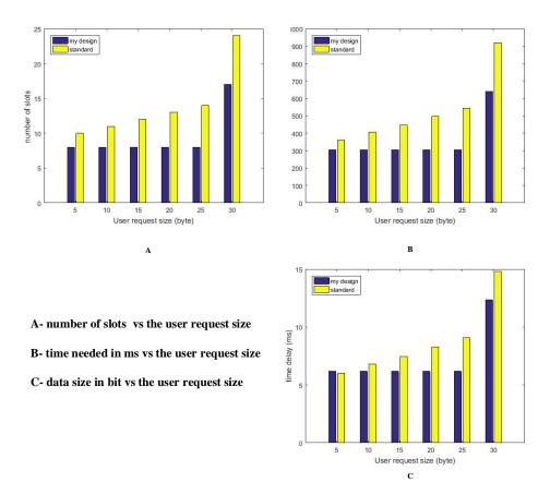
Figure C-2 Comparison Between Simulation Results of The Standard and The New Design for Uplink SF= 64
