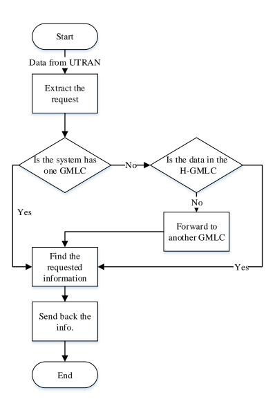
**Figure 5-10 Core Network Flowchart**
