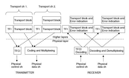
Figure 3-3 Interfaces Between Higher Layers and The Physical Layer
