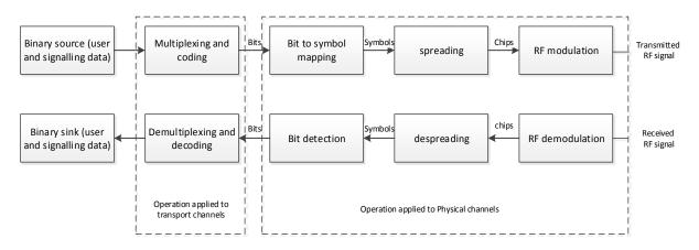
Figure 3-11 Simplified Transmission Chain in FDD Physical Channel
