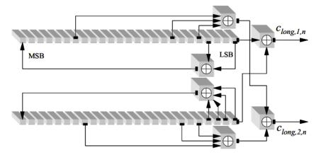
Figure 3-13 Long Scrambling Code for the Uplink
