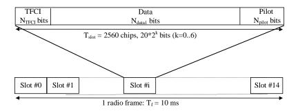
Figure 3-6 Radio Frame Structure of S-CCPCH
