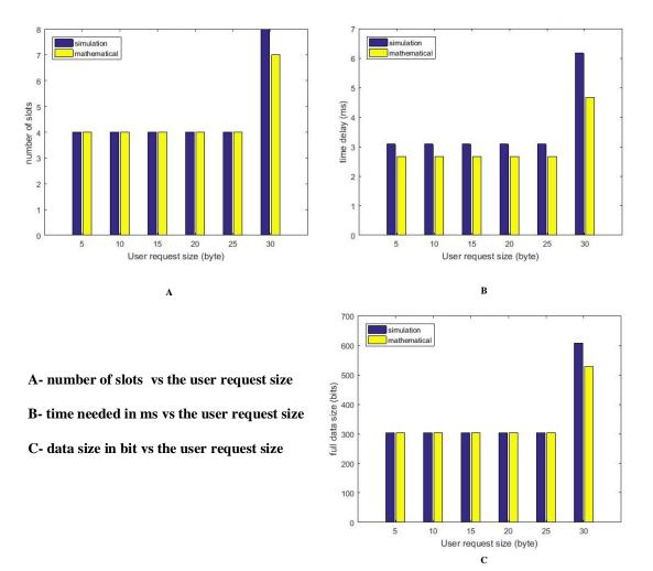
Figure B-1 Comparison Between The Mathematical Results and Simulation Result for Uplink with SF= 32
