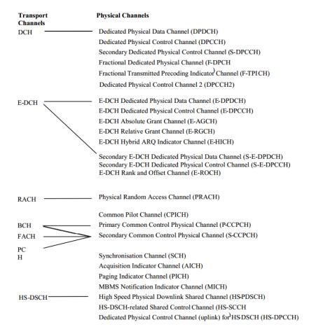
Figure 3-7 Transport Channels to Physical Channel Mapping
