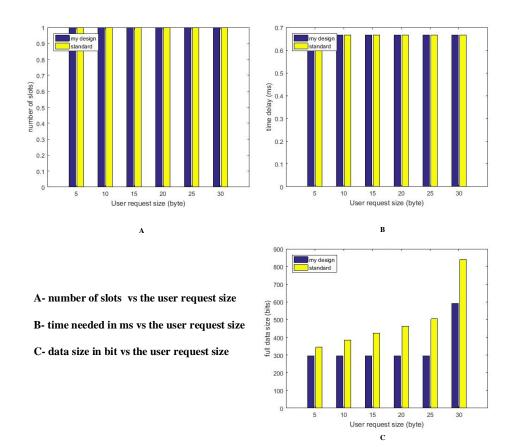
Figure C-5 Comparison Between Results of The Standard and The New Design for Downlink SF= 4
