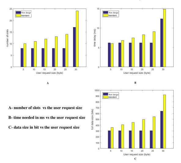
Figure 7-9 Comparison Between The Results of the 3GPP and The New Design for The Uplink SF= 64
