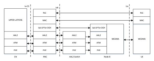
Figure 3-18 User Plane Protocol Stack for Circuit Switching [8, 68]
