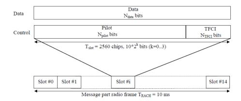
Figure 3-5 Frame Structure for RACH
