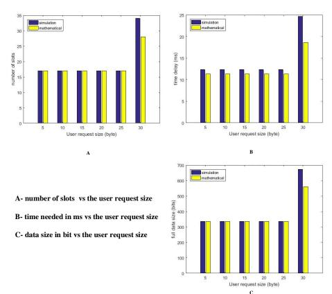
Figure B-3 Comparison Between The Mathematical Results and Simulation Result for Uplink with SF= 128
