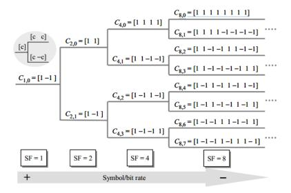
Figure 3-12 Tree Structure to Generate OVSF Codes
