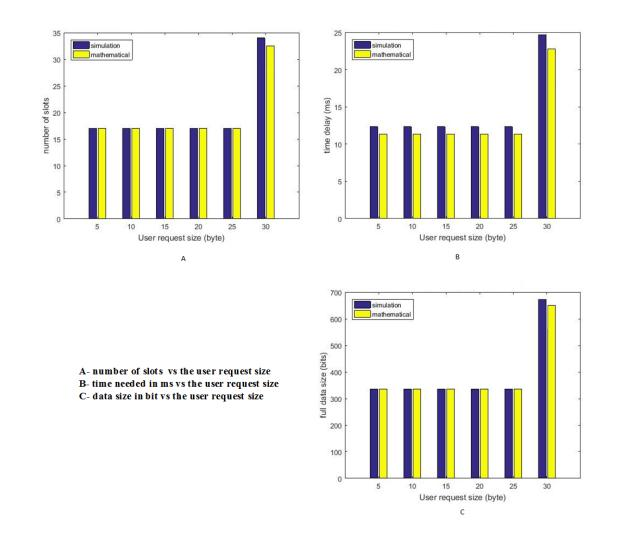
Figure 7-6 Comparison Between The Mathematical and Simulation Result for Uplink with SF= 128
