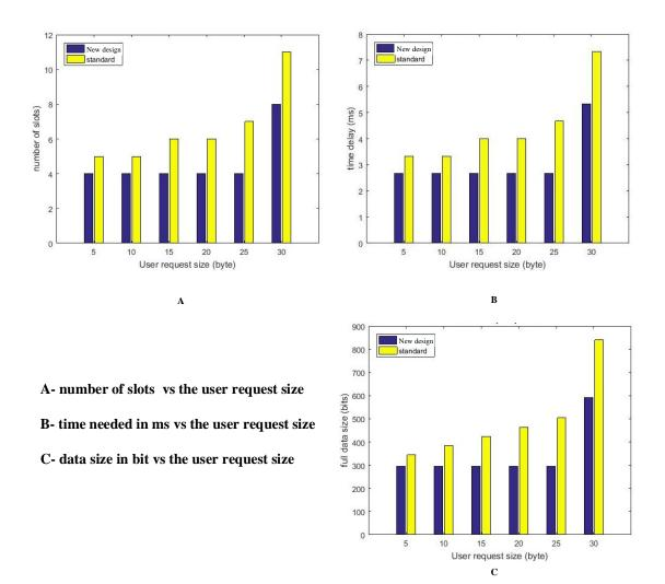
Figure 7-12 Comparison Between The Results of The 3GPP and The New Design for The Downlink SF= 64
