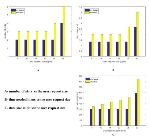
Figure C-8 Comparison Between Results of The Standard and The New Design for Downlink SF= 32
