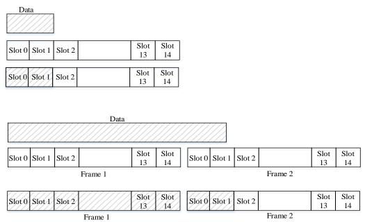
Figure 5-3 Data Mapped into Slots and Frame
