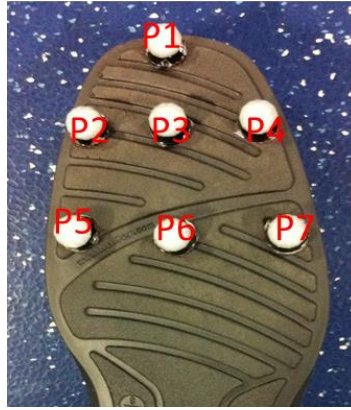
Figure 8: Sole marker setup to evaluate foot clearance. From Thies, Jones et al., (2011); Thies, Kenney, et al., (2011)
