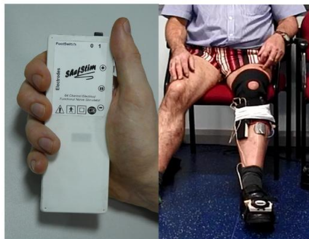
Fig. 6. ShefStim stimulator (left) being used by a subject during setup (right).
