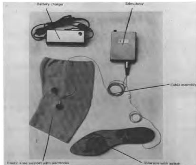
Figure 4: Ljubljana Functional Electrical Peroneal Brace. From (National Research Council, 1973)
