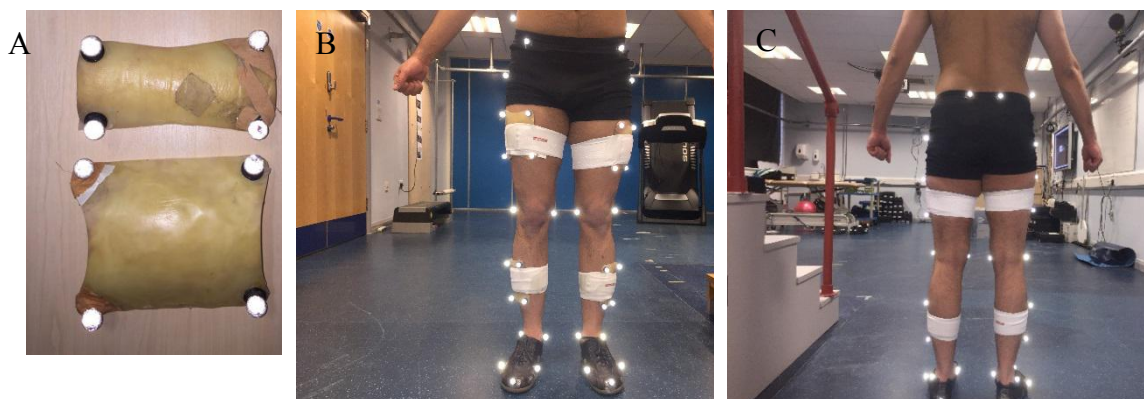
Figure 3- 8: Anatomical and technical reflective markers. (A) Passive reflective marker and cluster marker, (B) and (C) Location of the markers and clusters.
