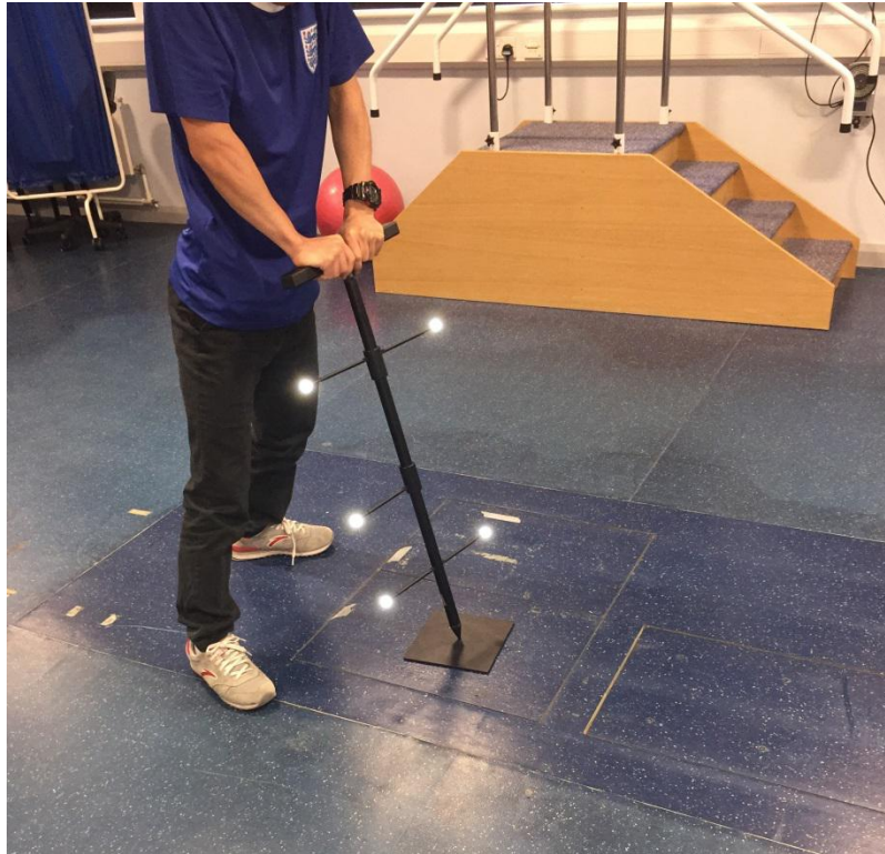
Figure 3-6: The CalTester rod was used to apply forces to the force plate
