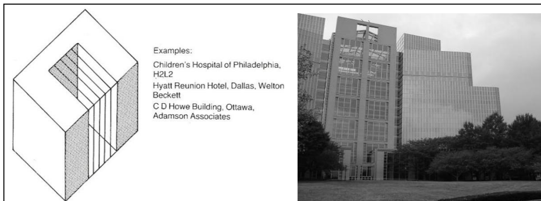
Figure 4. 10: Generic form of a three-sided atrium building on the left (Saxon, 1986) with an example of Hercules plaza, Wilmington as a three-sided example on the right (Bednar, 1986)
