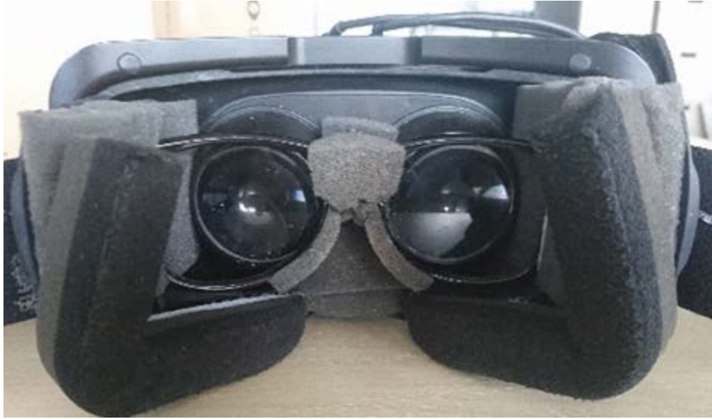
Fig.2. Custom Oculus Rift DK2 adapted for fNIRS
