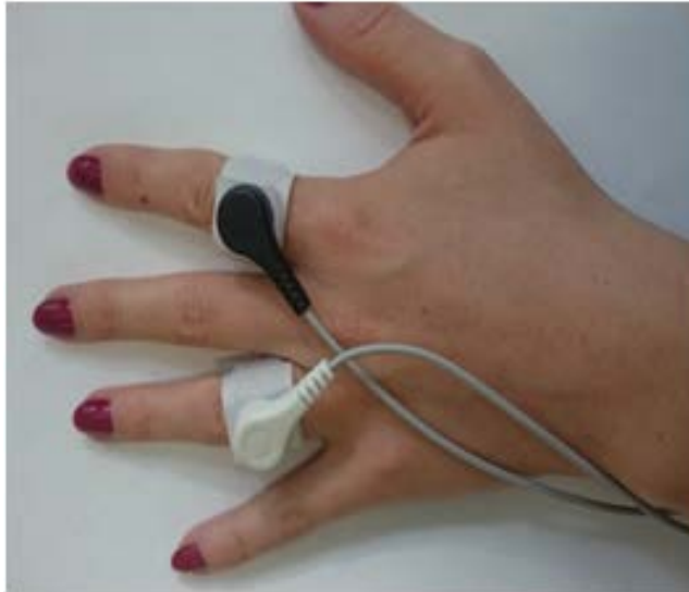
Figure 6 EduLogger GSR Sensor electrodes placement
