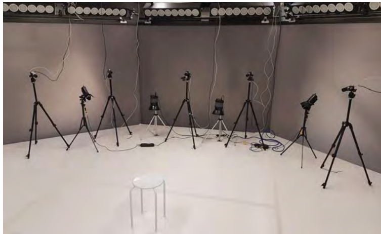
Figure 7.16: Five capture cameras and lighting provided significantly better frame rate and texturing for experiment 3. The walls around the Octave were also illuminated. The stool can be seen in the centre of the space
