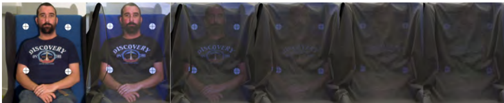
Figure 4.6: This is the projected image retro-reflected and photographed. The left hand image shows the bulk of the light from the image giving a clear view of the projected person. Very quickly each 5^\circ move to the right demonstrates a substantial falloff in the reflected light to that location. The human eye continues to resolve the image of a person beyond the right hand image in this example.
