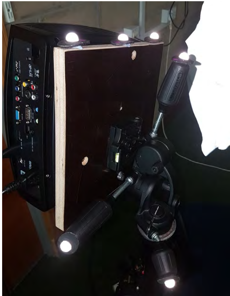
Figure 7.18: The Vicon retroreflective markers on the InFocus 1920x1080 projector show up clearly in the camera flash. This projector delivered 4x the pixel density of the other older units.
