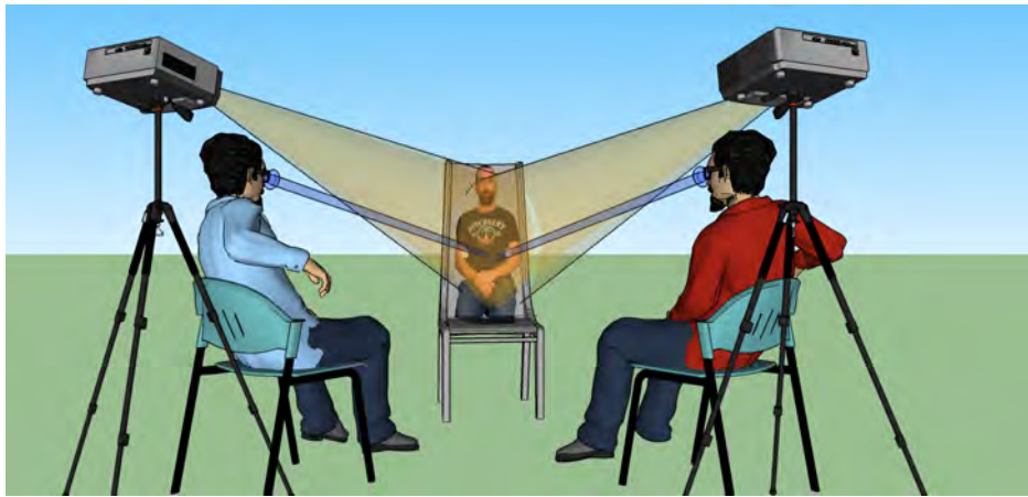
Figure 7.1: It is perhaps useful to remind the reader of how limited the previous system was. The two onlookers with spatially segmented views retro-reflected from Telethrone cannot move from their positions, and neither can the remote participant.
