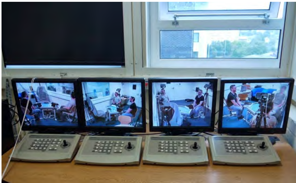
Figure 5.6: Observation suite camera control station. All of these feeds are steerable and zoomable using the controller, but are less visible to the users of the space as they are in enclosed ceiling domes. These were later synchronised and analysed for the gaze encoding alongside the two which captured through the one way mirror over the shoulders of the participants.
