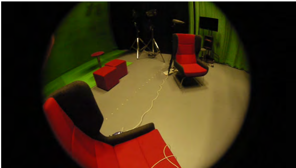
Figure 4.4: Controlled test set-up in MediaCity:UK studios. The sensor was moved along the line of markers on the floor which were set every 5^\circ from the projecting lens (seen at the top of the shot).
