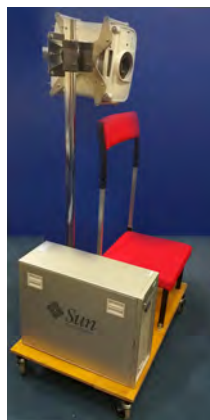
Figure 7.7: The prototype observing chair and projector are tracked for the view-point reconstruction but was not used in the experiment due to its weight. Instead, the computer shown was removed to a systems room.
