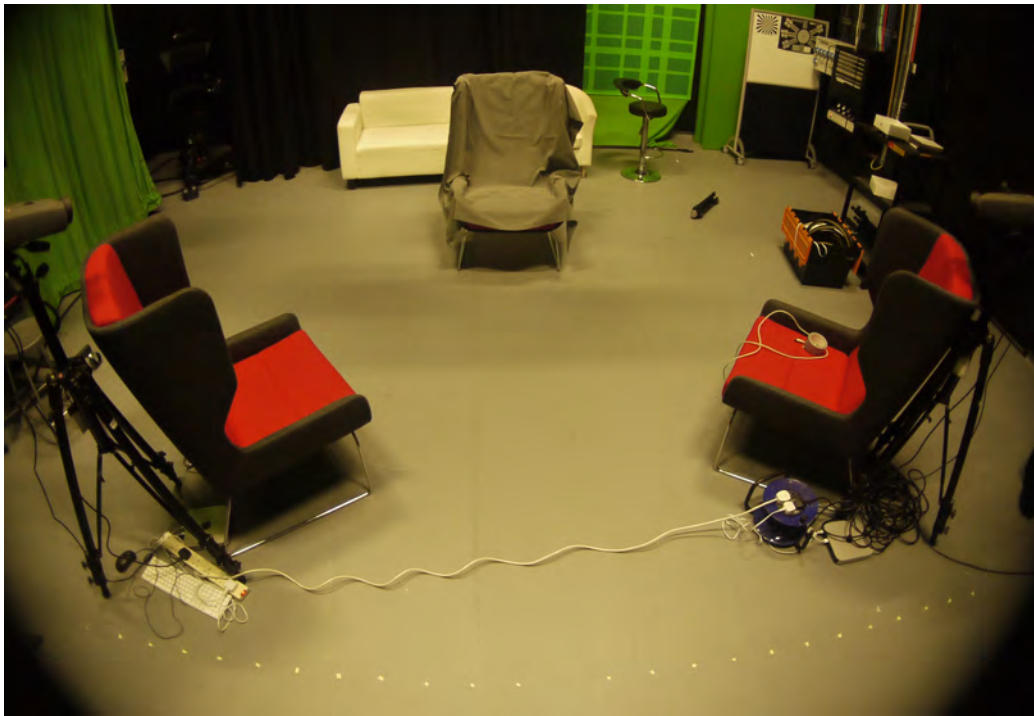
Figure 4.5: A clearer image of the light falloff set-up at MediaCity:UK with two stations. Both have an emitting projector. Multiple shots by 5^\circ deviation the lefthand projector toward the right hand projector show the blend between the two spatial segments.
