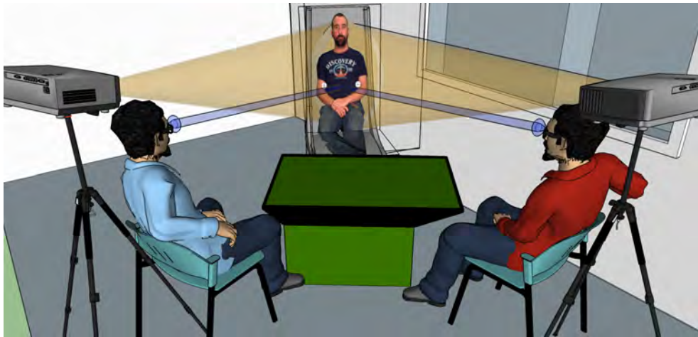
Figure 5.4: Light retro-reflecting from the two projectors back along the angle of incidence into the eyes of the associated onlookers. This is a gross over simplification of what’s going on optically with the reflected frustum, but is useful in that it makes clear that there are two segments of display here.
