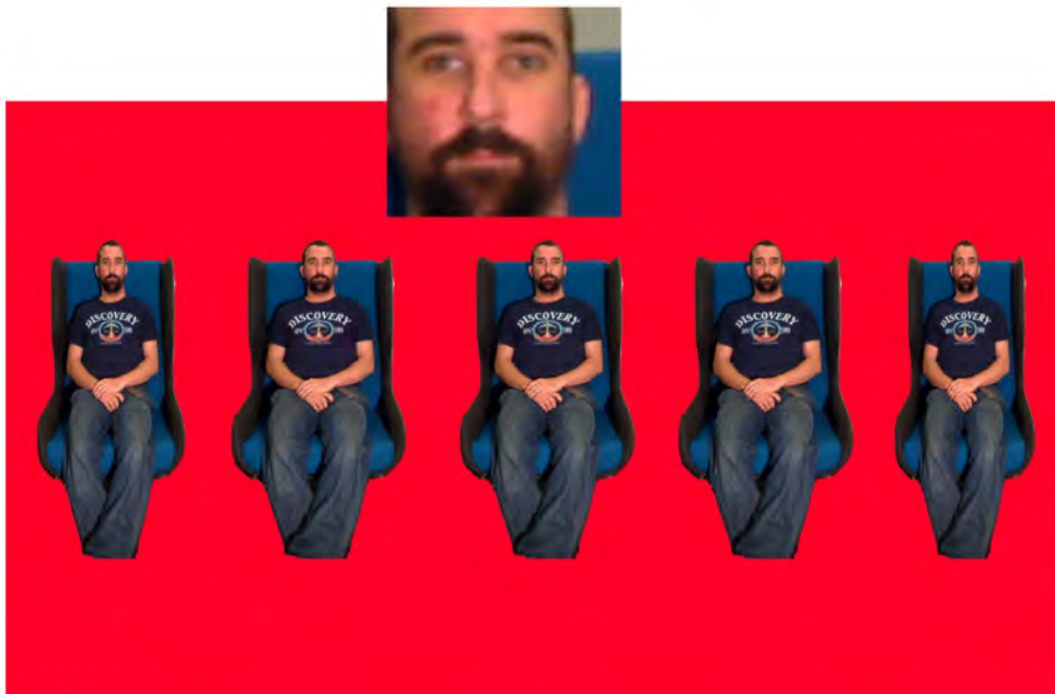
Figure 6.6: 130° projection frustum showing the distribution of pixels in the postulated 4k projection window (4096x2304 red area). The edge images are reduced by 5% as these are the adjacent seats to the projector and are more challenging and oblique targets. The whites of the eyes can still be made out as can be seen in the (actual pixels) zoom at the top of the image.
