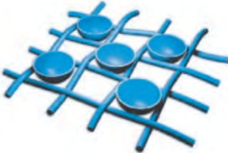
Figure 4.2: The Chromatte surface is a matrix of flattened micro lenses with an open front and reflective back surfaces. The lines are the stitches of the cloth which acts as a substrate for the lenses, (image credit reflecmidia)
