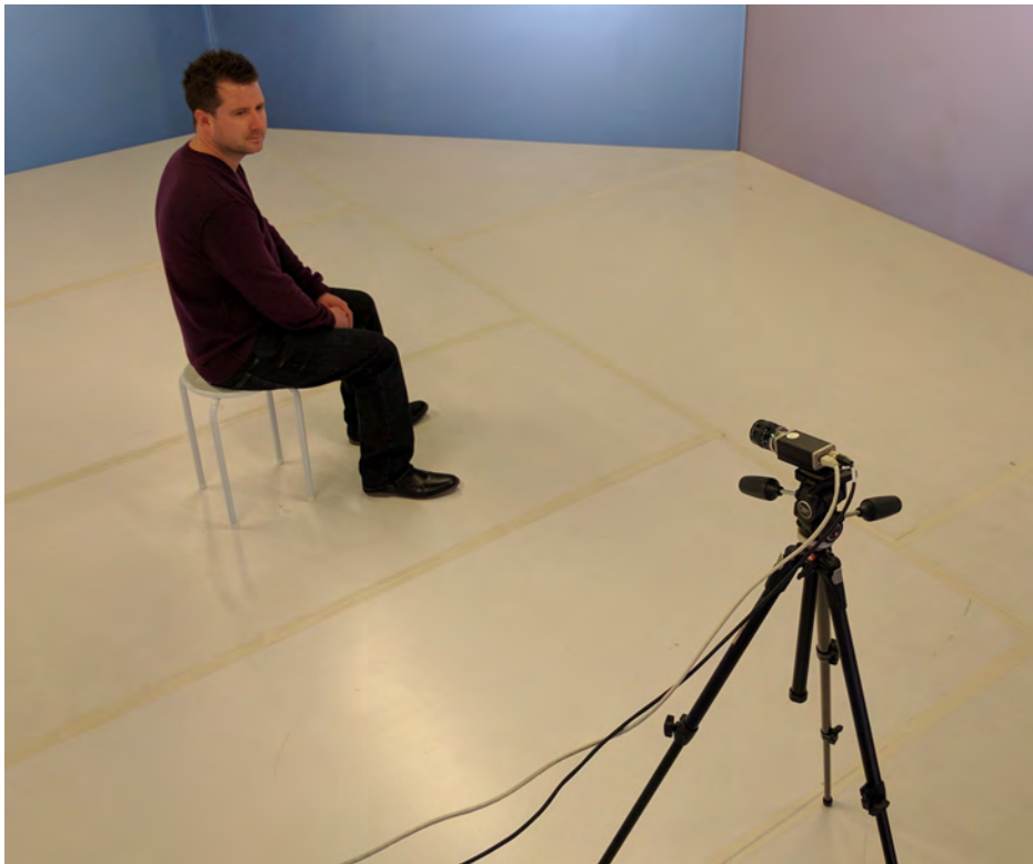
Figure 7.4: Capture of the subject in the Octave system for experiment 2. No additional lighting was used in this set-up and only a single camera was brought out of the ring in the ceiling space. The results were satisfactory as only a still image was required for this experiment. More light is needed only when moving 3D video is to be used.
