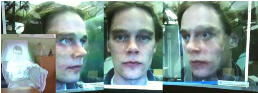
Figure 1: Early discussion and some testing across the group suggested that a chair (inset left) might be combined with retro-reflective material (seen demonstrating three isolated viewpoints of the same person). Rear projection of a micro-lensed material and lenticular sheets were trialled at this time with poor results.
