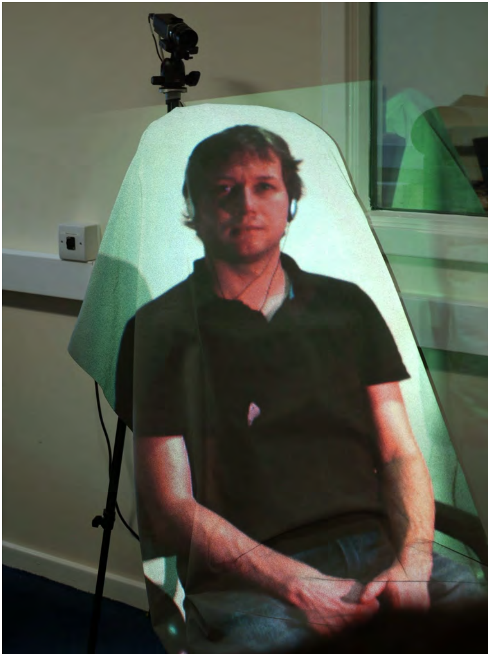
Figure 5.1: View from the participant station toward the Telethron. The remote participant whose gaze is toward the right hand side of the 60 inch TV seems to be looking toward the participant.
