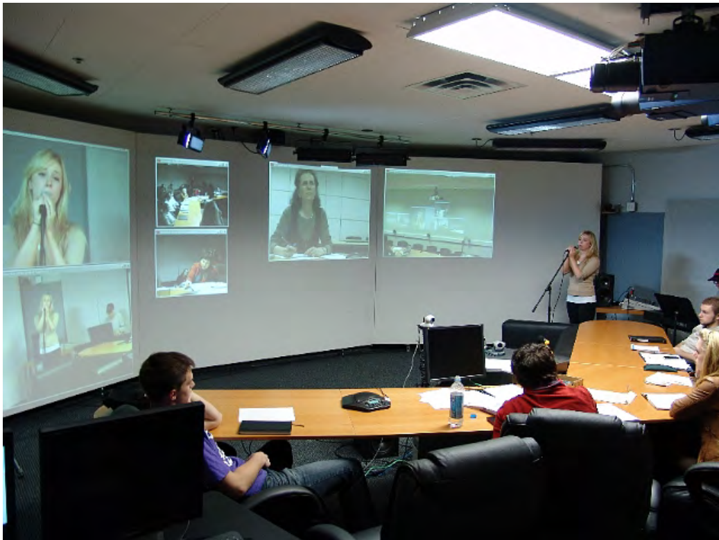
Figure 2.1: An access grid system. Such systems form a loose specification of ‘quality’ for aspects of the connection including latency, resolution, echo cancellation, etc. They are difficult to set-up and maintain and increasingly rare with Google searches for the term peaking in 2004 at 20 times the current level.
