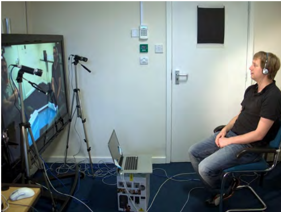
Figure 5.5: The remote user's station with IP cameras. As discussed elsewhere it can be seen that the cameras which capture the views for the two users on the right and left of the screen are not co-incident with their eyes being roughly 5^\circ apart.
