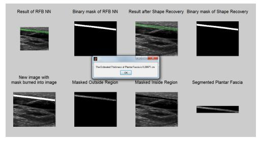
Figure C.7: RBF Neural Network Segmentation results with estimated PF thickness
