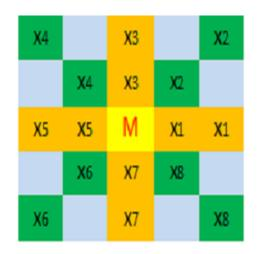
**Figure 2.11:** Diagram illustrating the neighbourhood pixels used in 5x5 kernel window of the Hybrid-Median filter. It shows 4 orientations including the central pixel M (Horizontal, vertical in yellow and two diagonals in green), the blue pixels are being ignored. It gives 4 output values (according to 4 orientations) that can be ranked separately using three iterations as in equation (2.41).
