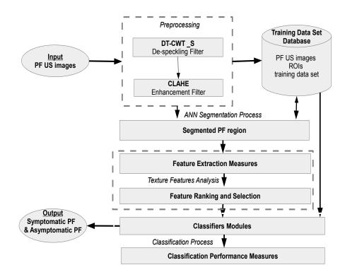
**Figure 5.2:** Flowchart illustrating the plantar fascia classification system based on a Texture features analysis and different classifiers modules
