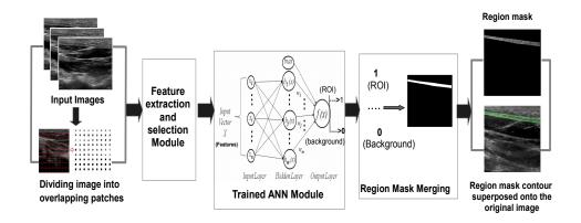
Figure 4.1: Block diagram showing ANNs approach to segmenting ROIs
