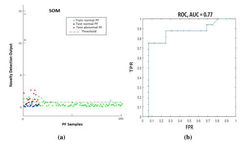
**Figure 6.7:** Results of the SOM model for PF dataset. The threshold is set to be 0.8 and represented by a horizontal line.
