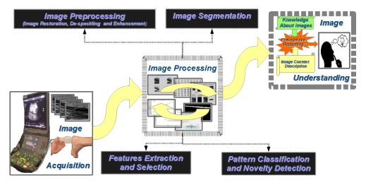
Figure 2.4: The main classes within image processing: Preprocessing, segmentation, features extraction and selection, pattern classification and novelty detection.
