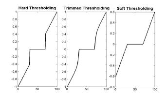
Figure 2.8: Trimmed thresholding compared to hard and soft thresholding (threshold T = 0.4 and  $\alpha = 7$ ).
