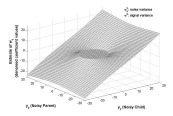
Figure 2.10: Bivariate shrinkage thresholding function.
