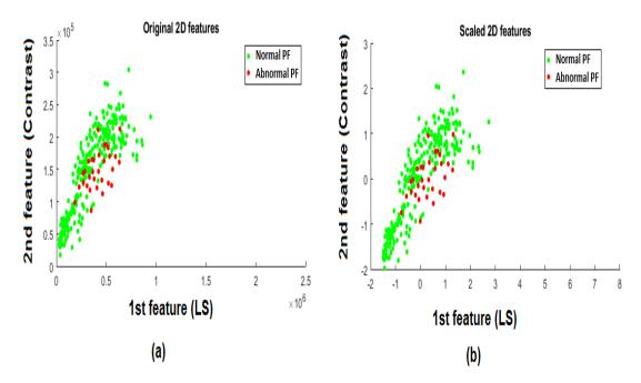
**Figure 6.3:** A 2-D plot representation of the top two selected features of 284 PF dataset (252 Normal and 32 Abnormal). Features of normal and abnormal PF samples are shown in blue and red, respectively. (a) PF features before scaling; (b) PF features after scaling (normalization). The plotting shows that the two selected features of the normal data and abnormal data lie in different range after scaling.
