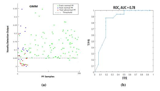
**Figure 6.5:** Results of a Gaussian Mixture Models (GMM) window estimator for PF dataset. The optimal threshold is set to 0,05 and represented by a dash-and-dotted horizontal line.
