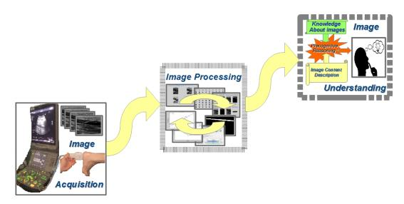
Figure 2.3: The three-step high-level medical image processing model: Image acquisition, image processing, and image understanding.
