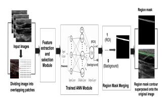
**Figure 5.4:** Block diagram showing ANNs approach for segmenting PF ROIs from PF US images dataset: (1) input dataset (preprocessed PF US input images with overlapping patches); (2) features extraction and selection; (3) PF image patches classification (PF and non-PF) using trained RBF-ANN classifier; (4) region mask formation(black background and white PF ROI); (5) region mask labelling and superposing.
