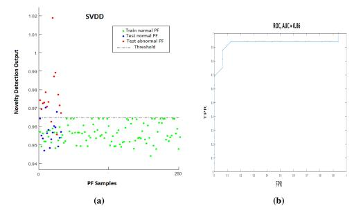
**Figure 6.8:** Results of a SVDD one-class classifier for PF dataset. The threshold is set to 0.965 and represented by a horizontal line. The analysis of the ROC curve for the SVDD approach confirms its high performance, as presented in Table 6.5
