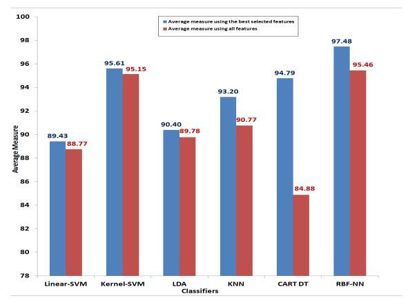
**Figure 5.12:** Average performance measure for different classifiers using different selected features (showing differences between classification models using the best selected features and others using all (40) features).
