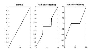
Figure 2.7: Hard and soft thresholding functions
