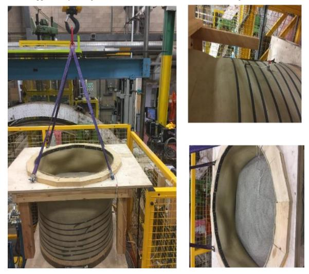
Figure 3-15 Soil container fixed on shaking table at Salford University
