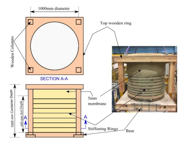
Figure 3-7 The soil container design
