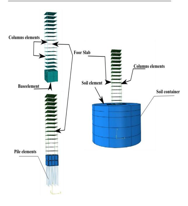
Figure 4-8 Numerical elements modelled by ABAQUS
