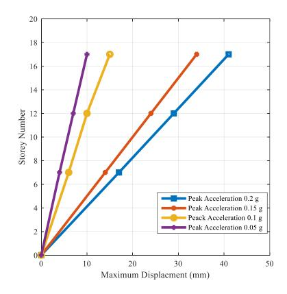
Figure 6-4 Effect of acceleration intensity on the maximum displacement (raft foundation)
