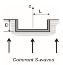
Figure 2-9 Embedded raft foundation (Stewart, 1999)
