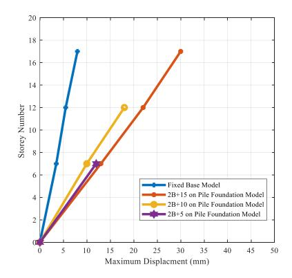
**Figure 6-9 Effect of structure height on the pile foundation**
