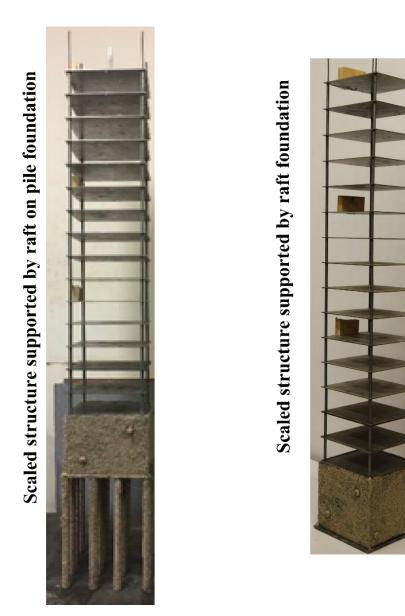
Figure 3-10 Constructed scaled model and foundation types
