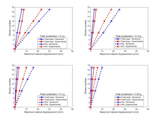
Figure 5-10 Structure on raft on pile foundation output
