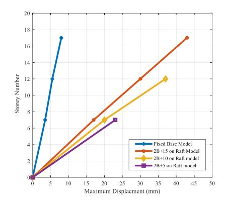
Figure 6-6 Effect of structure height on maximum displacement (raft foundation)
