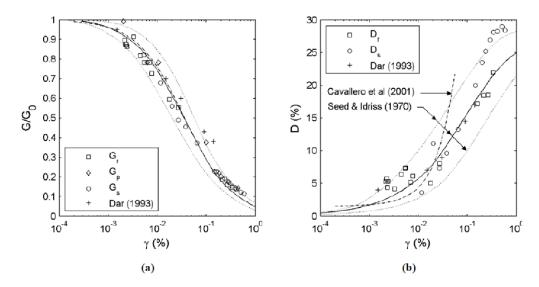
Figure 3-18 (a) The evolution of Shear modules G with shear strain γ (b) The evolution of damping Ratio D with shear strain γ (Seed et al. 1986)
