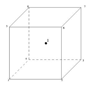
Figure 4-4 hexahedral C3D8R elements with integration point scheme (ABAQUS Documentation, 2013)
