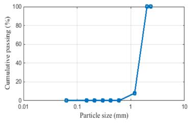
Figure 3-9 Sieve analysis of selected sand
