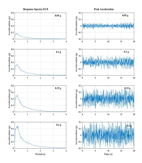
**Figure 3-11 Time – acceleration inputs**
