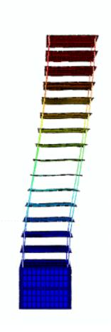
Figure 4-11 Fixed base numerical model by ABAQUS
