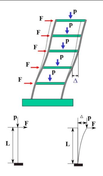
Figure 6-1 Configuration of P- $\Delta$  effect
