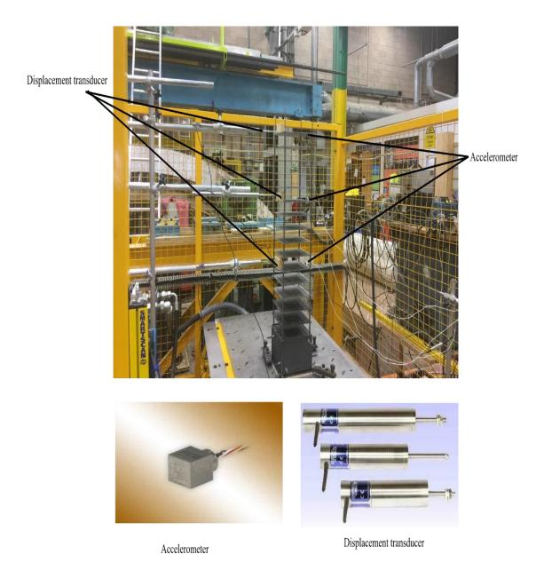
Figure 3-13 Fixed base shaking table test
