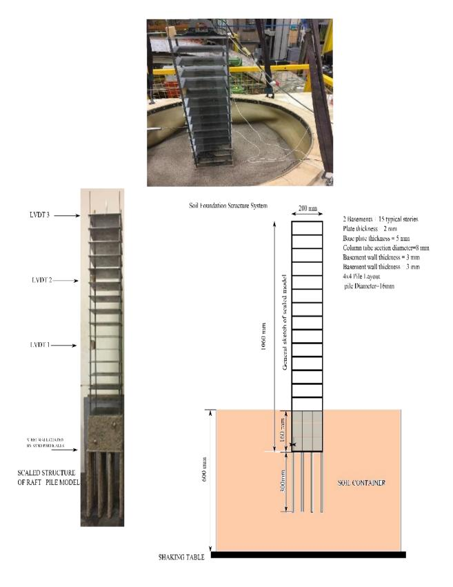
Figure 3-24 Soil foundation structure system details (raft on pile foundation)
