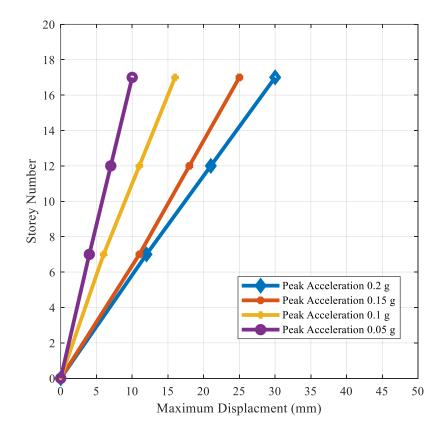
Figure 6-10 Effect of ground motion on maximum displacements (pile foundation)
