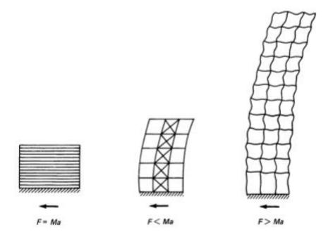
Figure 2-2 Schematic of seismic force representation(Taranath, 2009)
