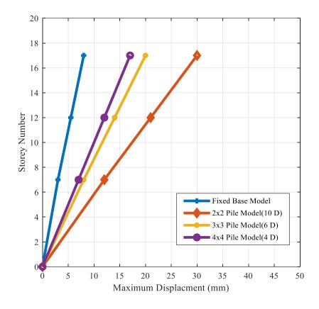
Figure 6-12 Effect of number of piles on maximum displacements
