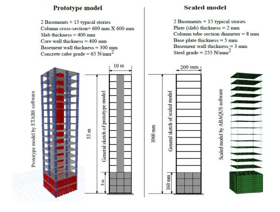
Figure 5-1 Detail of the prototype and scaled model
