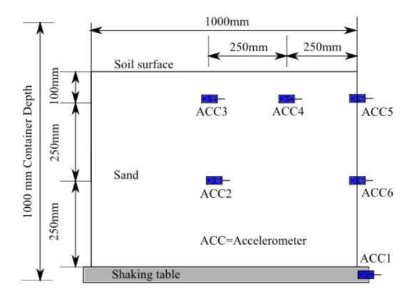
Figure 3-16 Layout of accelerometers
