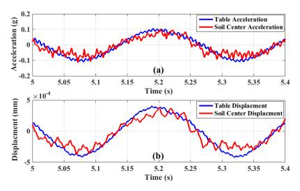
Figure 3-20 Measurement of time-acceleration and time displacement at the table and soil mass level
