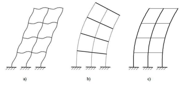
Figure 4-1 Shear deformation of multi-storey buildings under seismic force (Han and Cathro, 1997)
