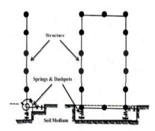
Figure 2-14 Soil model in lumped parameter methods (Bowles Joseph, 1996)
