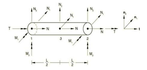
Figure 4-5 ABAQUS beam element B31 (ABAQUS Documentation, 2013)
