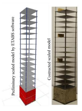
Figure 3-6 Scaled model design
