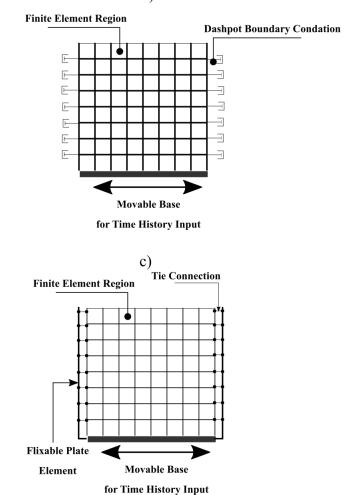
Figure 4-7 Numerical simulation of the soil boundary condition a) infinite boundary condition, b) dashpot boundary condition c) flexible plate element boundary condition
