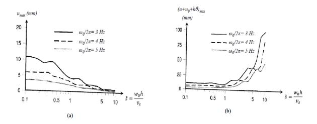
Figure 2-12 Response of the equivalent soil-structure system: (a) maximum structure demand, (b) maximum total displacement of the structure relative to the free field ground motion (Wolf and Obernhuber, 1985)
