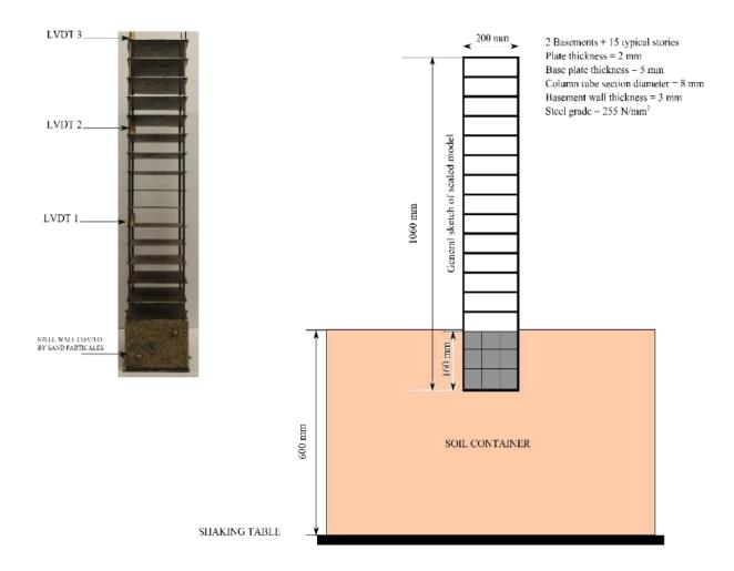
Figure 3-22 Soil foundation structure system details (raft foundation)
