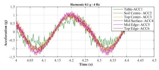
Figure 3-17 The effect of the container boundary of the soil response
