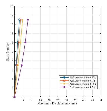
Figure 3-14 Fixed base experimental outputs
