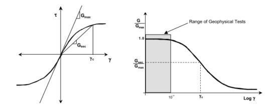
Figure 2-8 Stress-strain curve with a variation of shear modulus and modulus reduction curve (Tabatabaiefar and Massumi, 2010)
