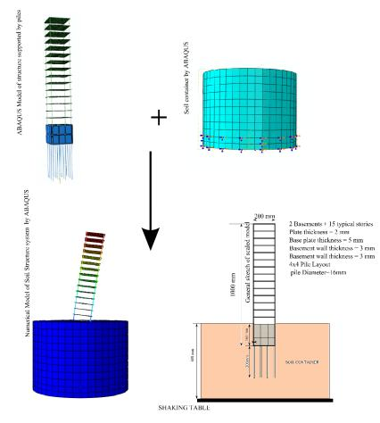
Soil Foundation Structure Interaction (Raft on Pile Foundation)
