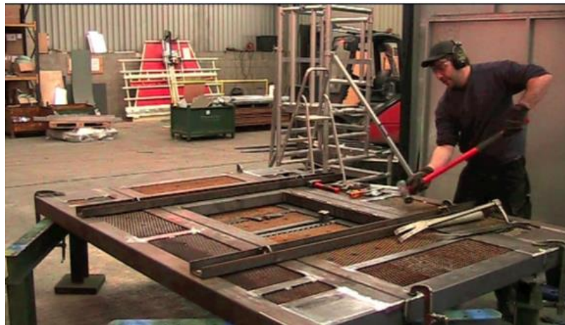
Figure 37 - Impact testing on roof panel at LPCB
