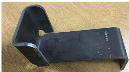
Figure 187 - New manufactured bracket
