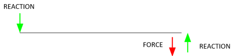
Figure 147- Beam representation of hinge system
