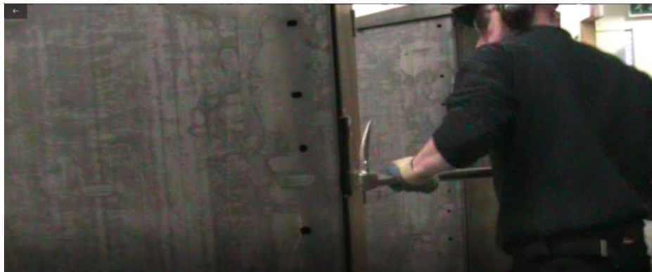
Figure 120 - LPCB lever attack
