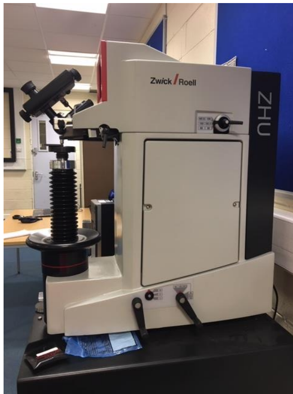
Figure 76 - Hardness test machine
