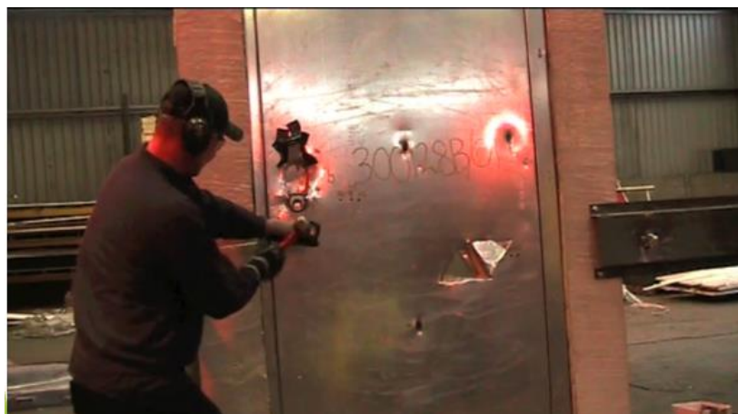
Figure 40 - Coupon creation at LPCB
