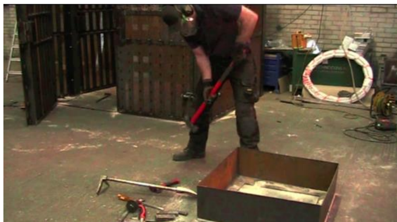
Figure 38 - Impact testing on Cover Frame at LPCB
