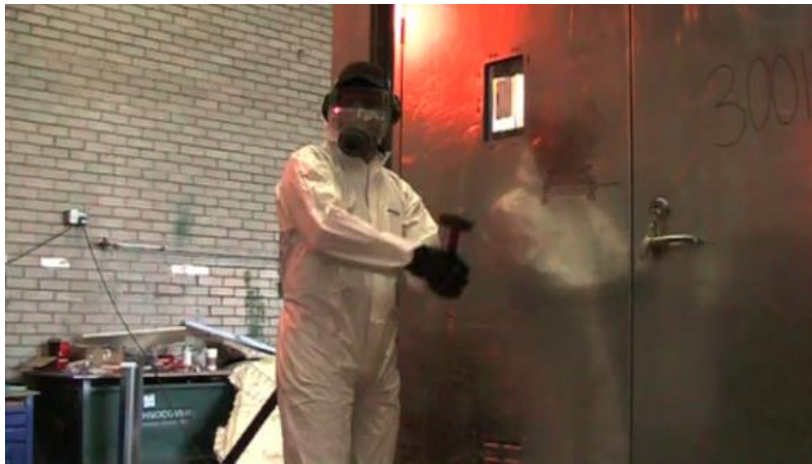
Figure 39 - Impact testing on glazing at LPCB
