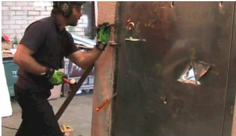
Figure 41- Leading edge attack at LPCB
