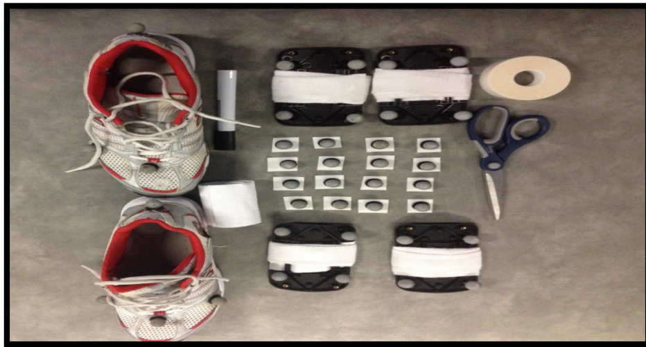
Figure 3- 5: The 3D motion system markers, clusters set-up for thigh and leg.
