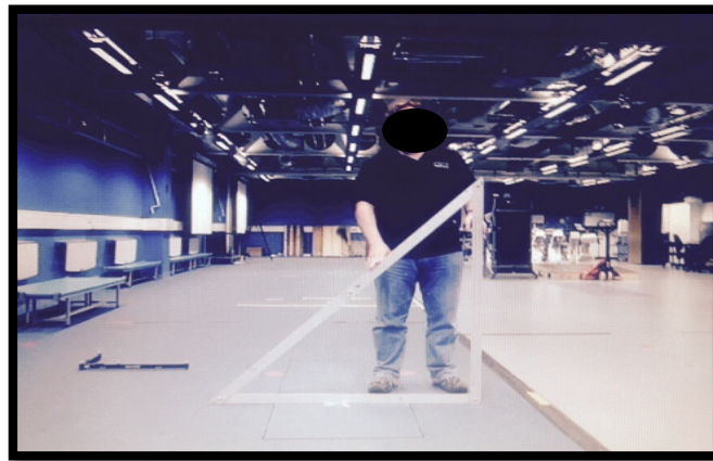
Figure 3- 1: Triangular Calibration frame.
