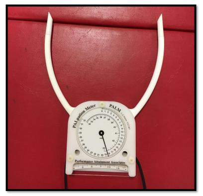
Figure 4-4: Inclinometer and it is main components (Palm meter).
