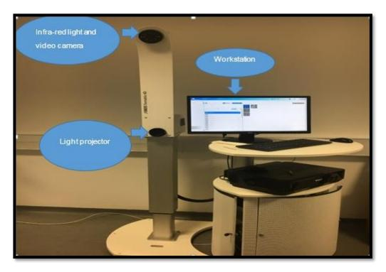
**Figure 4-6**: Diers system. This consists of a recording camera and light projector. The uneven back surface alters the straight projected light. The camera detects this distorted light from different angles of view and undertakes measurements.
