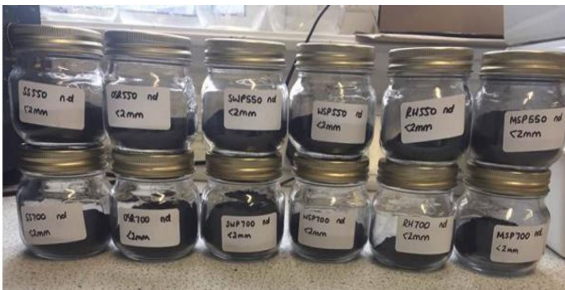
Figure 3.1 Feedstock and biochar samples as received from the manufacturer. A: Miscanthus straw pellet and biochar, B: Oil seed rape straw pellet and biochar, C: Rice husk and biochar, D: Sewage sludge and biochar, E: Softwood pellet and biochar and, F: Wheat straw pellet and biochar (Source: UK Biochar Research Centre, 2019).
