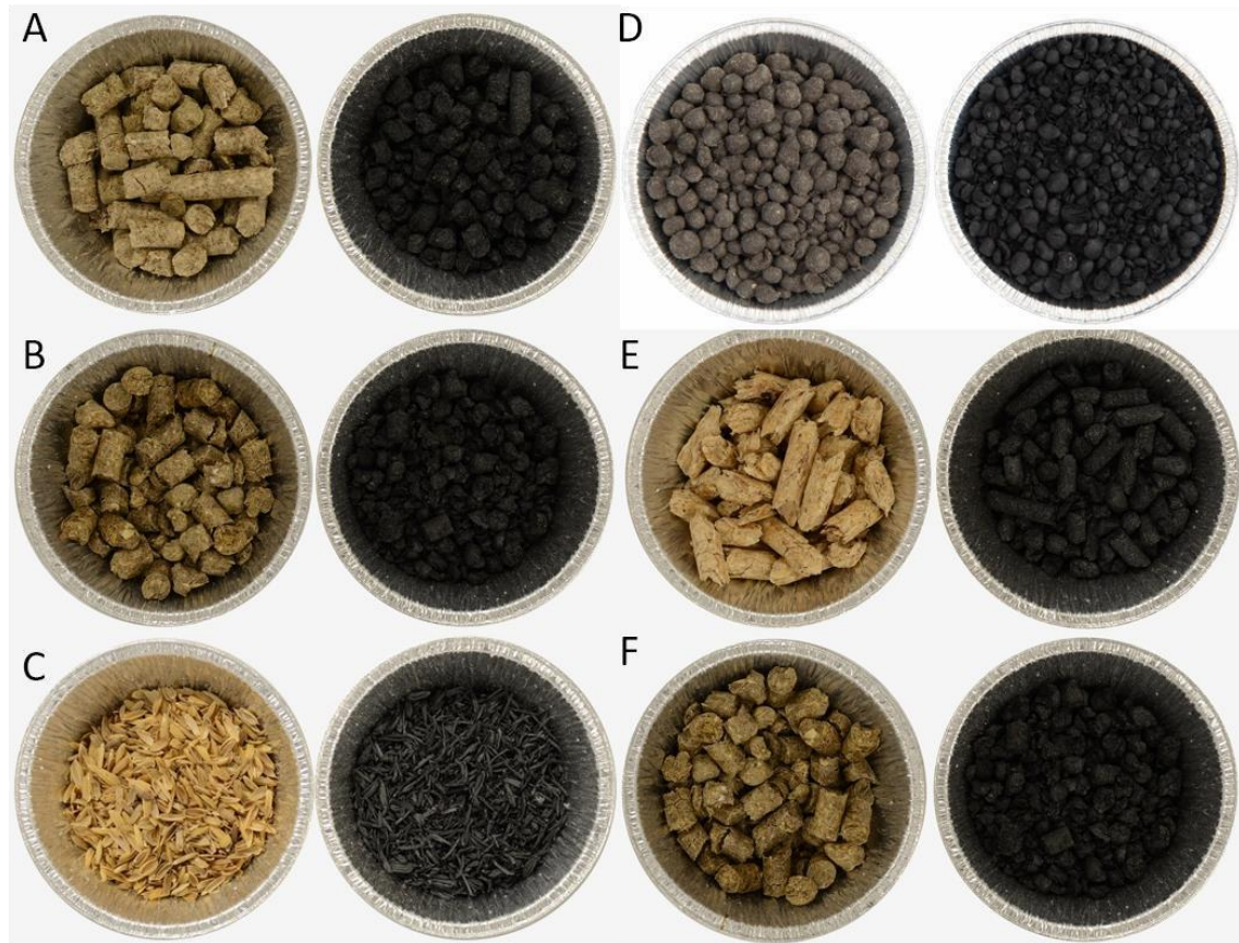
Figure 3.1 Feedstock and biochar samples as received from the manufacturer. A: Miscanthus straw pellet and biochar, B: Oil seed rape straw pellet and biochar, C: Rice husk and biochar, D: Sewage sludge and biochar, E: Softwood pellet and biochar and, F: Wheat straw pellet and biochar (Source: UK Biochar Research Centre, 2019).
