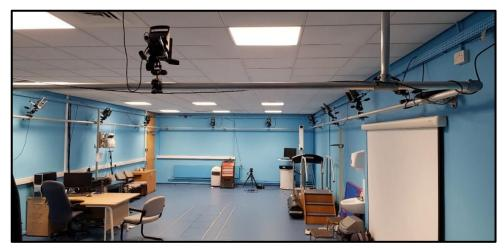
Figure 3.5: Stereophotogrammetry measurement system
