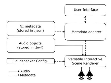
Figure 9.1 System diagram of the narrative importance control showing the flow of audio and metadata. Adapted from system diagram published in [378].
