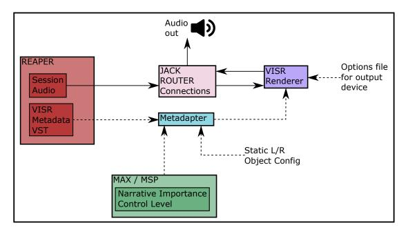
Figure 10.2 Flow diagram of the system used for Study Two, based on the end-user prototype described in Chapter 9 and the NI metadata assignment plug in shown in Figure 10.1.
