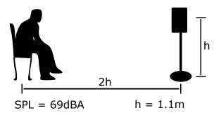
Figure 5.2 Experimental set up for Study One including participant location with reference to the loudspeaker, and height of the loudspeaker noted. Reproduction level set at the listening position is also given.
