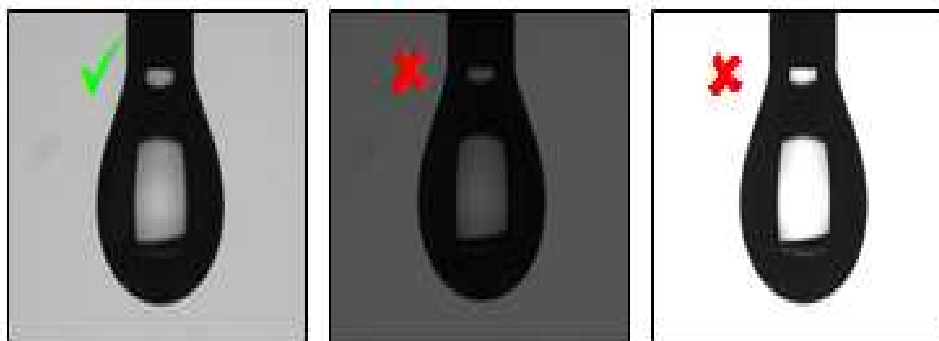
Figure 3.10: Drop Image with Suitable (A), Too Dark (B) and Too Bright (C) Background Illumination
