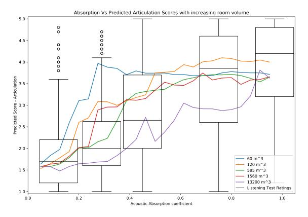
Figure 6.12: Generalisation test of the Articulation predictor on novel rooms and kick drum - Where coloured lines denote the room volume in test, x-axis shows the absorption coefficient used at the room boundaries and box plots show the distribution of Articulation scores across different absorption coefficients (where all room volumes are collapsed into this variance) to illustrate the deviation of generalised scores to actual subjective ratings.
