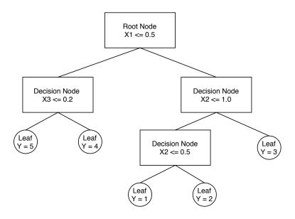
Figure 3.3: Simplified example of an arbitrary decision tree of depth 2. Where binary feature splitting is performed at inequalities in the decision nodes and predicted outputs are shown in the leaf nodes.
