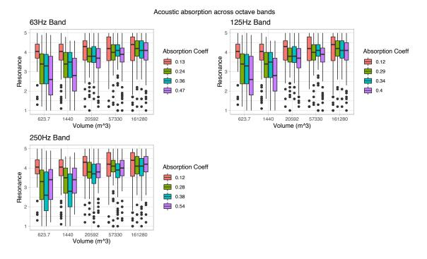
Figure 5.14: Illustrating the effect of varying the acoustic absorption coefficient between octave bands (split in each sub plot) - Where Resonance ratings are split between volume (x-axis) and acoustic absorption coefficient (coloured legend).
