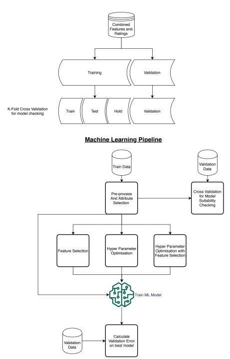
Figure 4.6: High level overview of the machine learning pipeline, where Data Splitting describes the process of forming a 80/20 train validation split of the combined feature and rating data and the further cross validation folds used for model suitability checking. And the machine learning pipeline which describes the modelling approach used to create different optimisations of the perceptual predictors.
