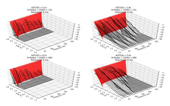
Figure 7.8: Convolved kick drum with room waterfall plot showing 4 rooms which either share the same Early Decay Time or Modal Density, represented as the number of modes under 250Hz. The Perceptual Modal Thresholds have been overlaid as a linear decay marked in red.
