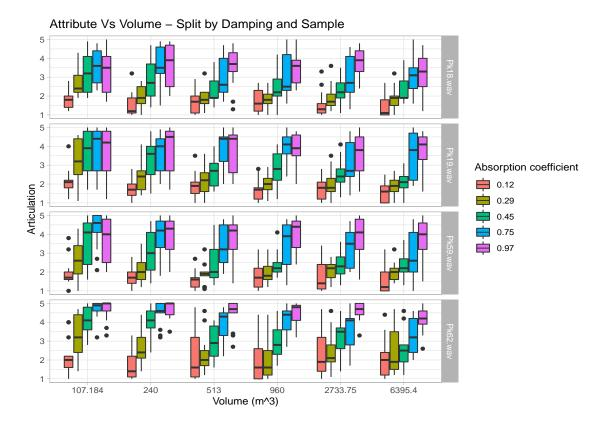
Figure 6.4: All second order interactions between variables and Articulation - Where sample is split across sub plot (denoted by the corresponding grey boxes), volume of room is shown in the x-axis and absorption coefficient is split by colour (shown in plot legend).
