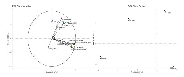
Figure 5.4: PCA of Kick drum space - Kick drums chosen for the subjective listening test, which are chosen from 4 corners of the factor plot (right). Where component 1 represents the decay characteristics of kick drum (denoted by decay based features on left hand variable plot) and component 2 represents features that describe the frequency content of the kick sample (denoted by the spectral based features on left hand variable plot).
