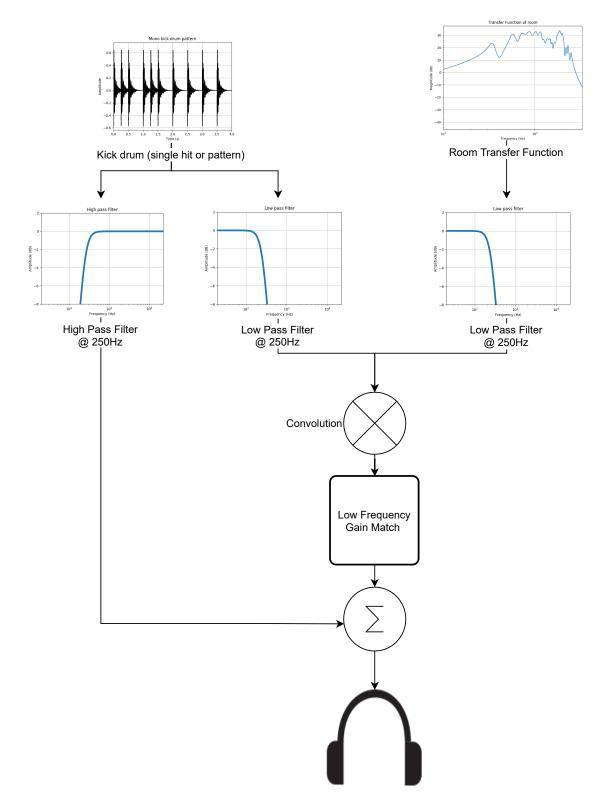
Figure 4.4: Diagram of the auralisation process adapted from (B. M. Fazenda et al., 2015) where output is an auralised kick drum between 20Hz and 250Hz with an assumed anechoic high frequency.
