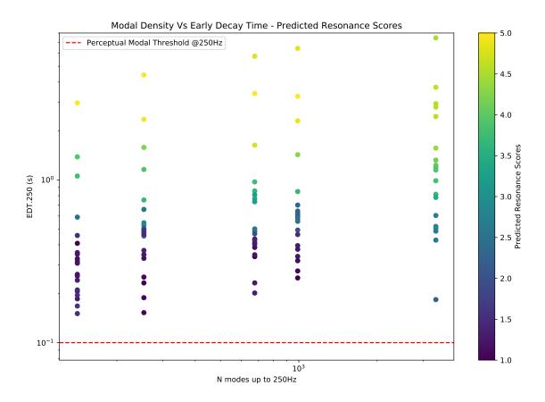
Figure 7.7: Use of the Resonance predictor to compare the effect of increasing modal density (described by the number of modes up to 250Hz x-axis) and Early decay time measured in the 250Hz octave band - Where the predicted Resonance score is coloured and shown in the colour map to the right of the plot.
