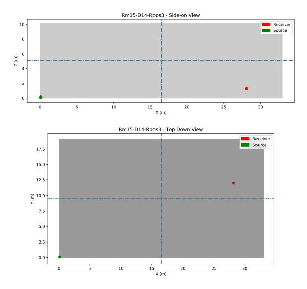
Figure 5.2: Source (shown in green) and Receiver (shown in red) positions of Rm15 showing the side-on elevation view and top down positional view where the dashed line denotes the half way point of the given axis.
