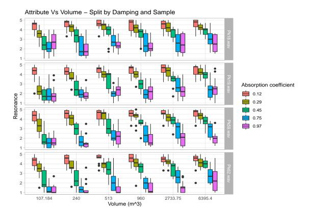
Figure 6.3: All second order interactions between variables and Resonance - Where sample is split across sub plot (denoted by the corresponding grey boxes), volume of room is shown in the x-axis and absorption coefficient is split by colour (shown in plot legend).
