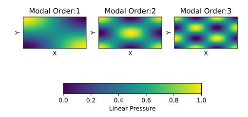
Figure 3.2: First 3 orders of a tangential mode across a 2:1 ratio rectangle demonstrating the pressure distribution across the horizontal axis - where the modal pattern is (1,1,0), (2,2,0) & (3,3,0).
