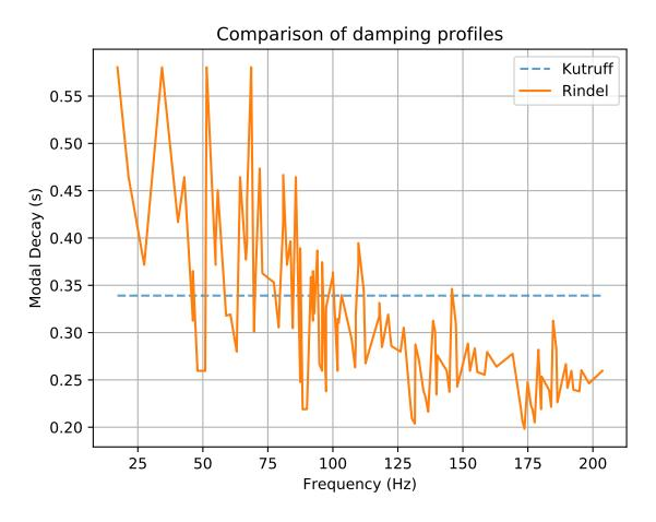
Figure 4.3: Comparison expressed in modal decay time between use of Equation 3.3 (Kutruff Method) and 3.11 (Rindel Method) - Assumed constant acoustic absorption coefficient of 0.5 across frequency range.
