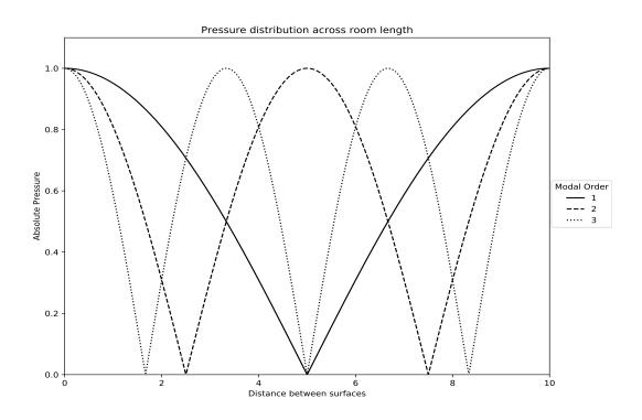
Figure 3.1: Modal pressure distribution across a single dimension illustrating the first 3 orders of resonance.
