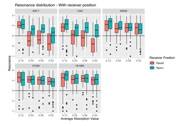
Figure 5.11: Illustrating the effect of including multiple receiver positions - where Resonance scores are split across volume  $(m^3)$  denoted in grey bar above each subplot and acoustic absorption coefficient of the room (x-axis). The black line denotes the mid point of the Resonance scale to highlight the skew of distribution in scores.
