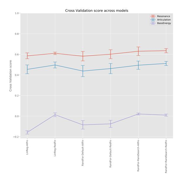
Figure 6.5: Checking the model suitability through cross validation k = 3 for Resonance (red), Articulation (blue), Bass energy (purple) across each model (shown in x-axis) - Where each point denotes the mean cross validation score across folds and the upper and lower bound lines denotes the standard deviation across all folds.
