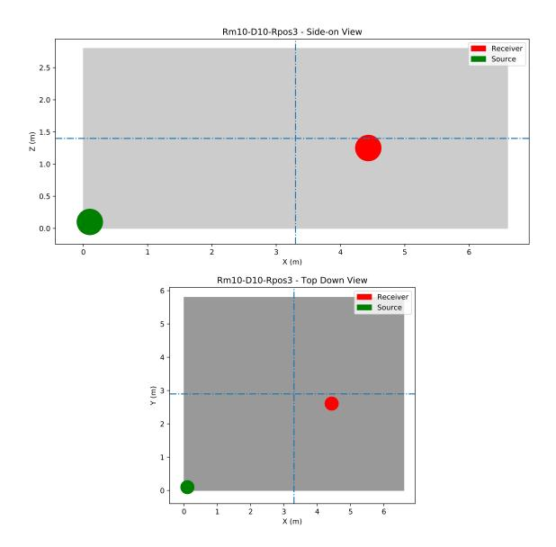
Figure 5.1: Source (shown in green) and Receiver (shown in red) positions of Rm10 showing the side-on elevation view and top down positional view where the dashed line denotes the half way point of the given axis where the source is placed in a corner and receiver is placed at an estimated seated head height of 1.25m at a random offset from the 2/3rds position in the room (simulated FOH position).
