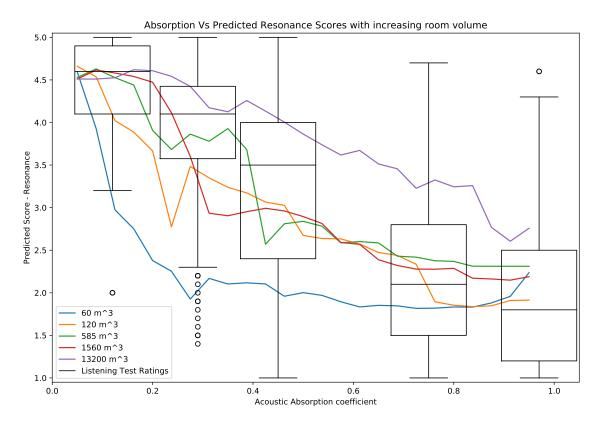
Figure 6.11: Generalisation test of the Resonance predictor on novel rooms and kick drum - Where coloured lines denote the room volume in test, x-axis shows the absorption coefficient used at the room boundaries and box plots show the distribution of resonance scores across different absorption coefficients (where all room volumes are collapsed into this variance) to illustrate the deviation of generalised scores to actual subjective ratings.
