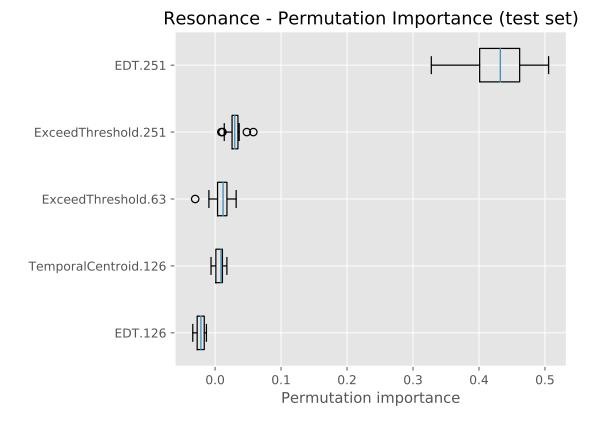
Figure 6.9: Random forest permutation importance for the reduced feature Resonance model shown for the validation/test data set.
