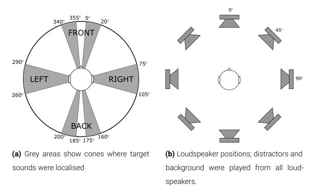
Figure 4.3.: Target locations and experimental setup.
