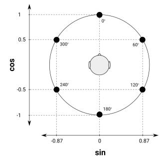
**Figure 5.5:** Positions of the secondary target and their corresponding sine and cosine values. Positive sine values indicate positions to the right of centre, and negative – to the left. Positive cosine values represent positions in front of the listener, negative – in the rear.
