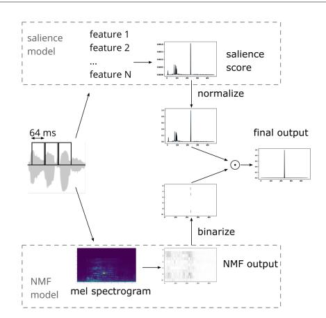
Figure 11.1.: Structure of the model combining NMF with auditory salience.
