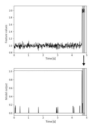
**Figure 10.2:** Example of how the salience score was calculated. Top: artificial feature (sound type) with added noise; the context builds an expectation of a sound of one type (value 1), but in the last 200 ms, the sound type is changed (value 2). Bottom: output of the salience model; the single-number score is the maximum over the duration of the distractor – here, the grey area.
