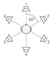
**Figure 3.2:** Loudspeaker setup in the listening room.
