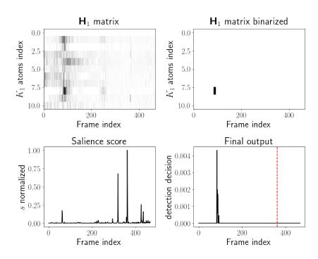
**Figure 11.2.:** Results for a gunshot event over a residential area background, with a loud car passing in the first half of the file. Top row:  $H_1$  matrix from the NMF model. Bottom left: salience model output *s*. Bottom right: final output of the model, from which an event is detected for any value larger than 0. Red dashed line shows the position of the target event. Even though it was correctly recognised by the salience model, the combined models do not detect it.
