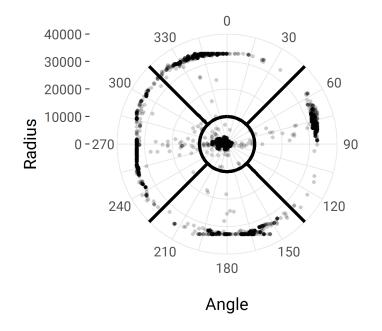
**Figure 4.6:** Raw joystick movement data for one of the baseline experiment participants. Each dot is one joystick position sampled at regular time intervals. The dots are partly transparent, so the darker the region, the more data points there are. Solid black lines show how the space was divided into quadrants and the centre area.
