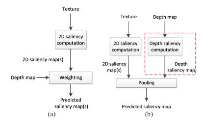
Figure 9.4.: Comparison of depth-weighting and depth-salience models, from Wang et al. 2013
