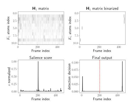
**Figure 11.3.:** Results for a gunshot event over a cafe/restaurant background. Top row:  $H_1$  matrix from the NMF model, before and after binarization. Bottom left: salience model output *s*, after normalization. Bottom right: final output of the model, from which an event is detected for any value larger than 0. Red dashed line shows the position of the target event, which was correctly recognised by the salience model, but not the NMF model.
