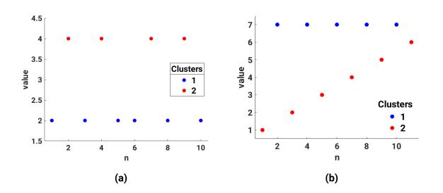
**Figure 10.3.:** Examples of two simulated feature streams, with colours indicating the result of GMM clustering. Each point represents one feature value at a time n, and colours show how they were assigned to one of two clusters. Notice that in panel b), the two clusters have different shapes – something that a k-means algorithm could not correctly deal with.
