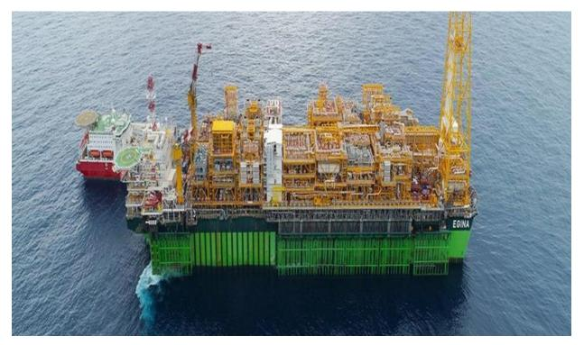
FIGURE 2.7 EGINA FPSO Anchored at location Offshore
