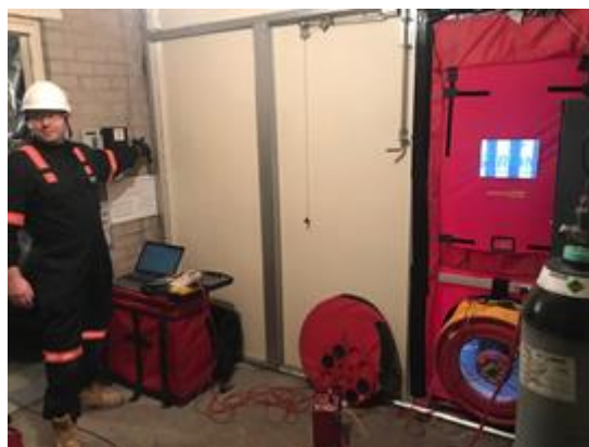
Figure 27: Blower Door Test Underway
