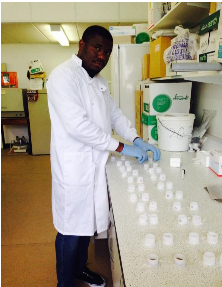
Figure 3.7. Laboratory soil sample preparations for XRF analysis
