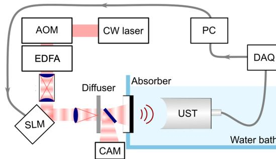
**Figure 1.** Diagram of the PAWS system. To simplify the diagram, passive optics are omitted including: a polarizer and half-wave plate prior to the SLM; lenses after the diffuser; neutral density filters on the camera.
